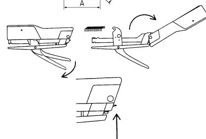
**Loading system:** top loading; pull-down the handle,
