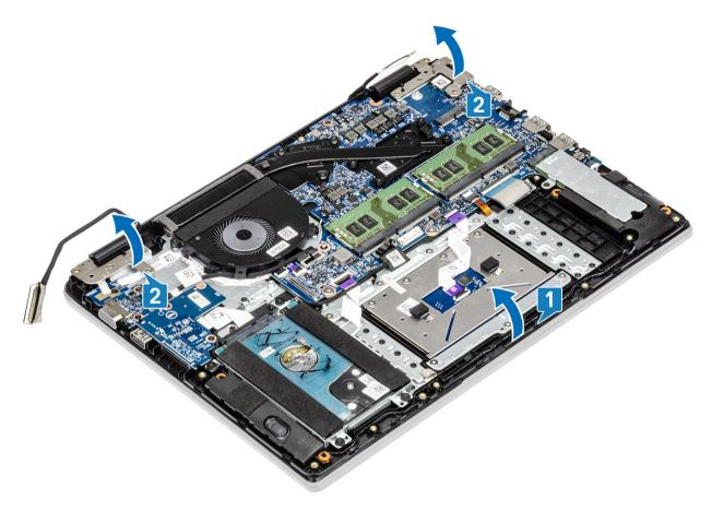
7 Slide and remove the palmrest and keyboard assembly off the display assembly.
