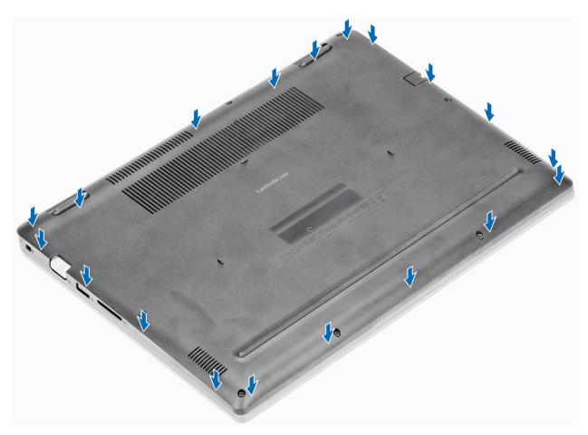
2 Tighten the nine captive screws that secure the base cover to the palmrest and keyboard assembly.
