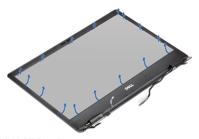
3 Lift the bezel off the display assembly.
