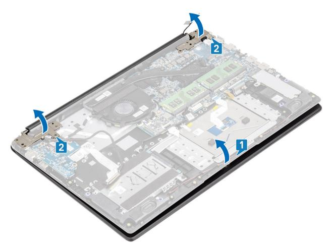
7 Slide and remove the palmrest and keyboard assembly off the display assembly.
