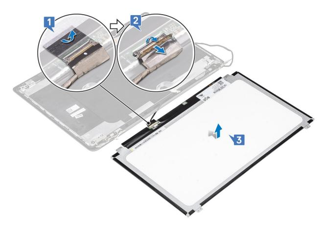
NOTE: Do not pull and release the Stretch (SR) Tapes from the display panel. There is no need to separate the brackets from the display panel.
