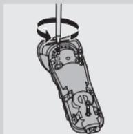
**6** Undo the three screws in the sealed power unit by means of a screwdriver on the back of the shaver.
