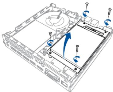
2. Insert your HDD or SSD into the storage bay, then secure it with four (4) screws.
