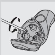
**3** Undo the two screws in the hair chamber.
