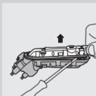
**8** Remove the power unit cover with a screwdriver.
