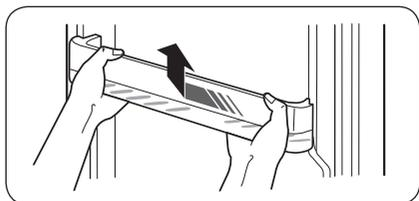
Slightly lift up and pull out the door guard.
