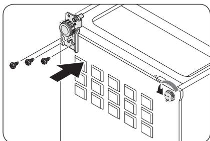
1. Lay down the refrigerator with care. Then, remove the screws from the **bottom hinge** on the right side and the **levelling leg** on the left side, respectively.
