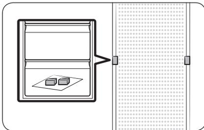
1. Open the door and locate the provided spacers (x2).
