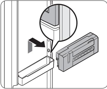
2. While holding the marked area on either side of the Slim Ice Maker unit with both hands, lift up the unit and pull out to the front.
