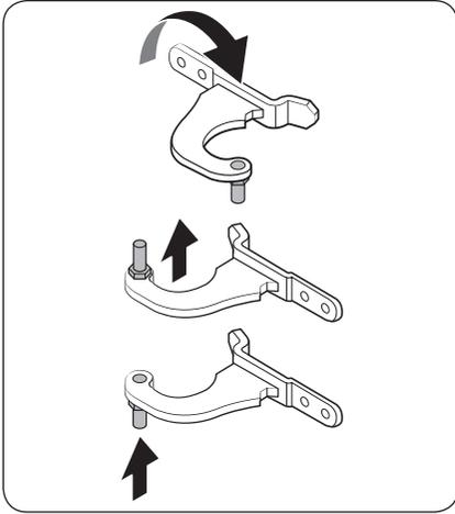
3. Remove the **shaft** from the **top hinge**. Then, reassemble the **shaft** as shown.
