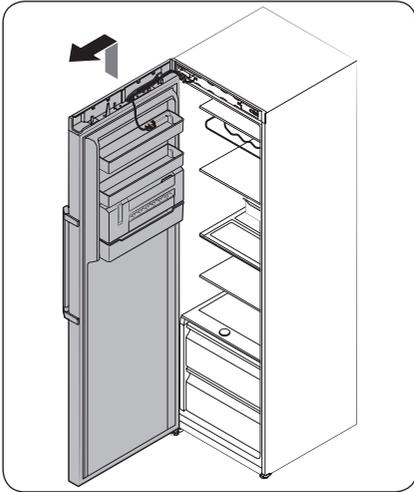
3. Disconnect the connectors on or around the freezer door. Loosen the screws from the **top hinge** to remove.
