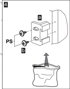
**Note:** Installation step for 2, screws for connecting top plastic part should not be screwed very hard, because of moving the plastic part easily left or right side.
