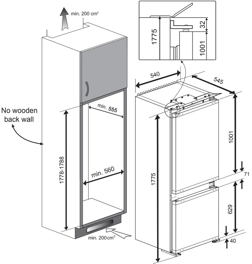
The back wall of the wooden cabinet must be left open completely to kitchen wall in order to allow sufficient air circulation to cool down the condenser unit for energy efficiency.
