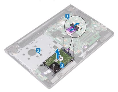
Disconnect the interposer from the hard-drive assembly.
