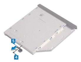
Carefully pull the optical-drive bezel and remove it from the optical drive.
