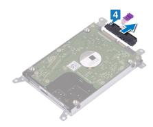
Remove the four screws (M3x3) that secure the hard-drive bracket to the hard drive.
