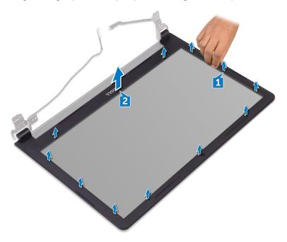
2 Remove the display bezel off the display back-cover and antenna assembly.
