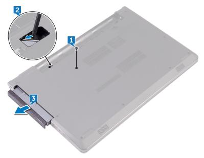
Remove the screw (M2x3) that secures the optical-drive bracket to the optical drive.
