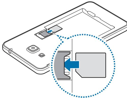
► **Dual SIM models:** Insert the SIM or USIM card with the gold-coloured contacts facing downwards.
