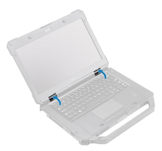
Place the brackets[1] and secure it using two 'M2.5\*5' on either sides [2].
