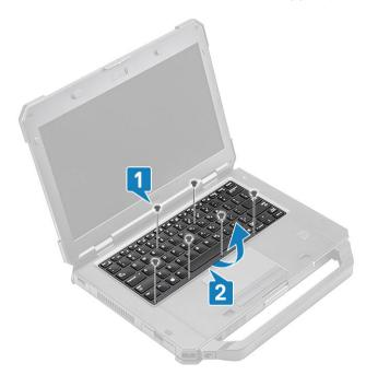
4 Slide the keyboard slightly [1] towards touch pad and flip it over inclined over the LCD panel [2].
