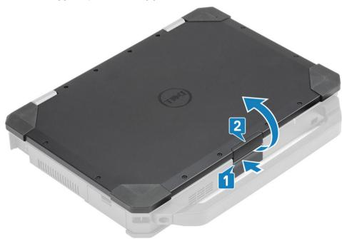
2 Keep LCD lid open at an obtuse angle and insert the hinge covers from front until it clicks in its place.
