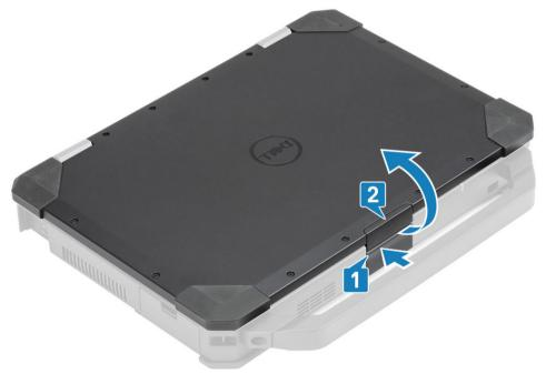
5 Hold the LCD lid at an obtuse angle and push the hinge covers from the rear end to remove it from the computer.
