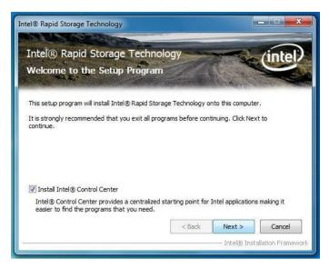
Please remember to check on the "Install Intel® Control Center" otherwise the user graphical interface RAID management software would not be install. Click 'Next' to continue the installation. Once the installation completes, user will get the "Intel Rapid Storage Technology" icon on the Windows task bar:
