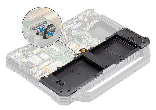
Remove the five 'M2.5\*3' [1] and nine 'M2.5\*5' [2] screws securing the battery bay to chassis and lift to separate the battery bay [3] from the computer.
