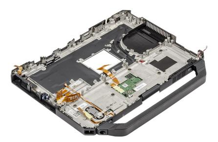
NOTE: See the order details to determine the exact specifics of subcomponents defined in the Bottom Chassis Assembly.
