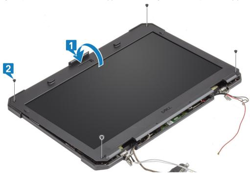
4 Install the 12 'M2.5' screws to secure the back cover to the LCD with bezel assembly.
