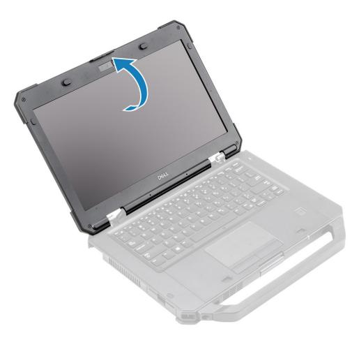
6 Loosen the two screws on hinges [1] to separate the LCD assembly from the computer [2].
