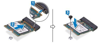
4 Align the screw holes of the M.2 thermal shield with the screw holes on the palm-rest assembly and system board.
