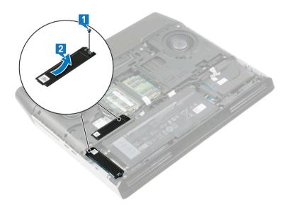
3 Remove the screw (M2x3) that secures the M.2 2230 card to the palm-rest assembly.
