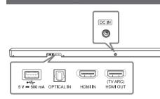
· · Connect to the AC adapter. ····Connect to a USB device. OPTICAL IN -·····Connect to an optical device. ······Connect to device with HDMI OUT. (TV ARC) HDMI OUT ..... Connect to a TV.
