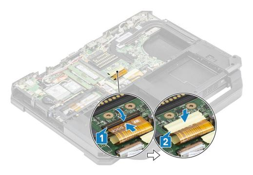
3. Secure the antennae cables along the routing channels [1] and connect the antennae cables on RF passthrough connectors [2].
