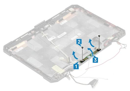
4. Peel off the insulation tape [1] and disconnect the EDP cable connectors [2].
