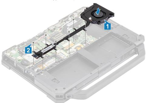
3. Tighten the three  $^{1}M2*3^{1}$  screws on the fan case [1] and connect the fan cable [2].
