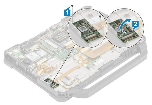
**6.** Remove the tape [1] and disconnect the Smartcard Reader FPC connector [2] from the USH board.
