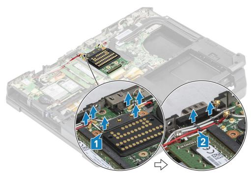
5. Remove the two 'M2.5\*5' screws [1] and separate the docking board assembly from the chassis [2].
