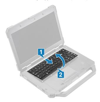
5. Remove the four 'M2\*3' screws [1] on the keyboard cover and remove it from the computer [2].
