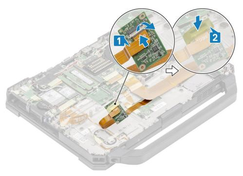
3. Install the two  $^{1}M2*3^{1}$  screws [1] and turn over the USH board to secure it to the chassis [2].
