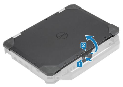
5. Hold the LCD lid at an obtuse angle and push the hinge covers from the rear end to remove it from the computer.
