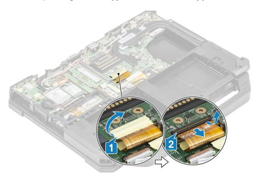
**4.** Disconnect the antennae cables from RF passthrough connectors [1] and unroute the antennae cables [2] from the routing channels on the dock assembly.
