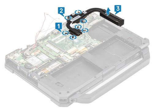
i NOTE: Discreet and UMA bases have different types of heatsink assembly.
