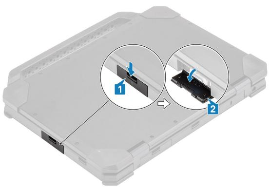
2. Withdraw the stylus out of the slot.
