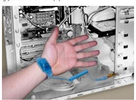
Figure 8. Bonding Properly
