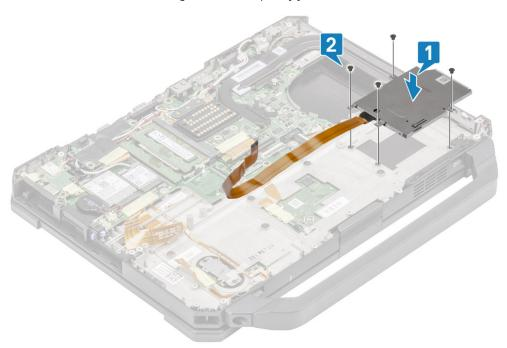
2. Connect the Smart Card FPC on the underside of the USH board [1] and secure it using a piece of tape [2].
