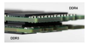
Figure 5. Thickness difference
