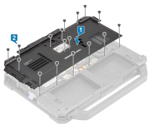
3. Tighten the two 'M2.5\*6' screws [1] in the rear I/O space and close the rear and left I/O doors [2].
