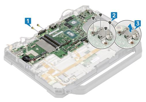
**14.** Remove the eight 'M2.5\*5' screws [1] and single 'M2\*3' screw [2] on the system board and remove the system board from the chassis [3].
