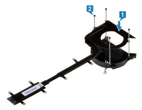
2. Install the PCle heatsink assembly [1] in the computer and install the seven 'M2.5\*5' screws on heat sink pipe [2].
