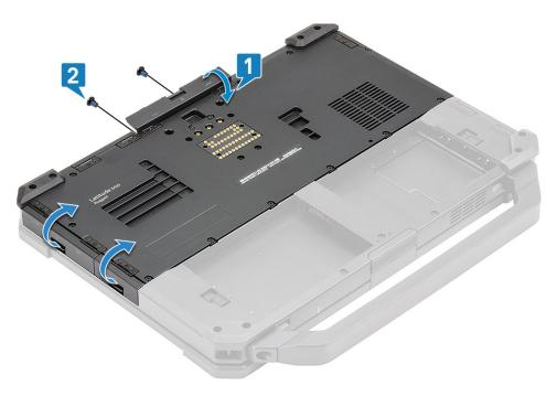
**4.** Remove the 17  $^{\prime}$ M2.5\*5 $^{\prime}$  screws on the bottom chassis cover [1] and remove the bottom chassis cover [2] from the computer.
