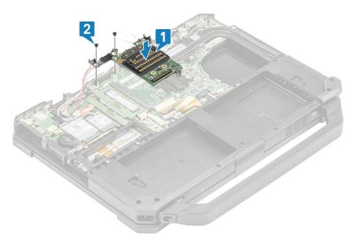
2. Connect the dock FPC [1] and secure it using a piece of tape [2].
