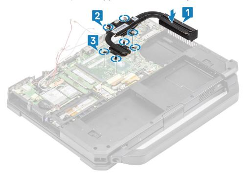
3. Route the antennae cables along the routing channel on the heatsink pipe.
