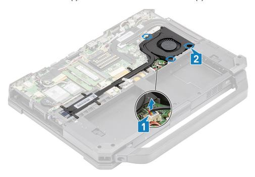
**4.** Loosen the seven 'M2.5\*5' screws [1] from heat sink pipe and remove the PCle heatsink assembly from the computer [2].
