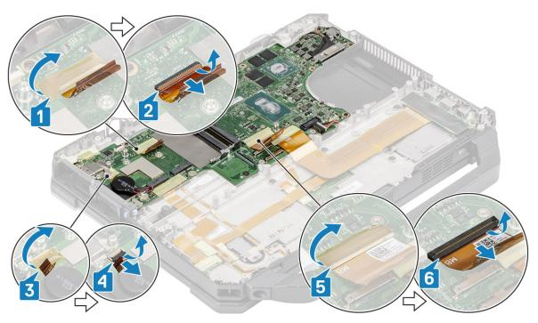
7. Peel off the tape [1] and disconnect the left I/O board FPC connector [2] from the system board.
