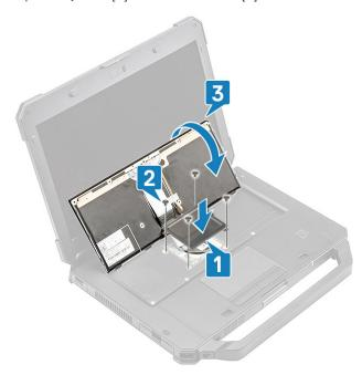
$\textbf{5.} \quad \text{Slide the keyboard towards LCD [1] to align it to screw holes [2].}$
