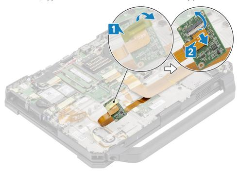
7. Loosen the four  $^{1}M2*3^{1}$  screws [1] and remove the smart card [2] reader from the computer.
