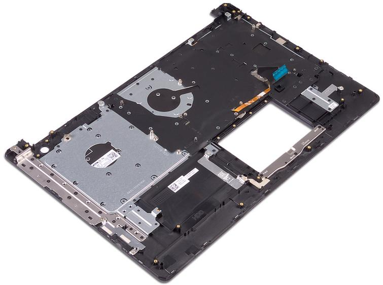
Place the palm rest and keyboard assembly on a flat surface.
