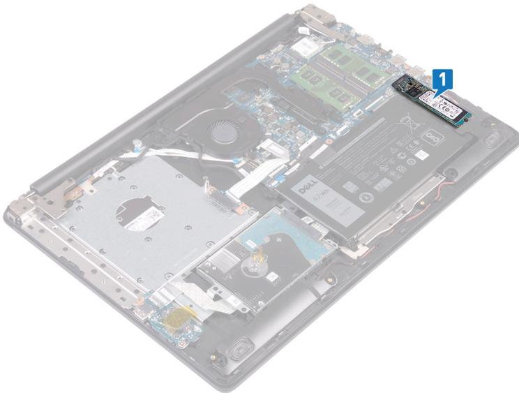
**① NOTE:** If available, remove the thermal shield before removing the solid-state drive/Intel Optane.
