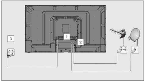
For digital satellite stations (DVB-S/S2) plug the cable of satellite antenna into the antenna socket RF IN-S2 on the television set:
