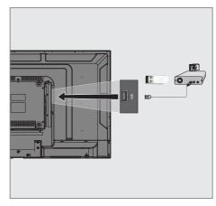
1 Connect the »USB« interface of the television and the corresponding socket on the data device (external hard disk, digital camera, card reader or MP3 player) using a USB cable.
