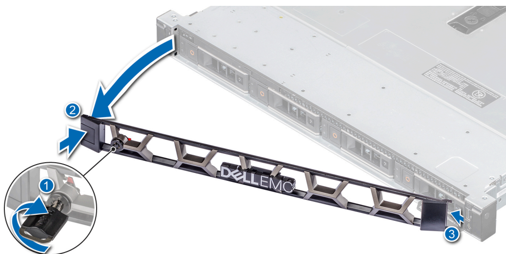
Figure 9. Removing the front bezel
