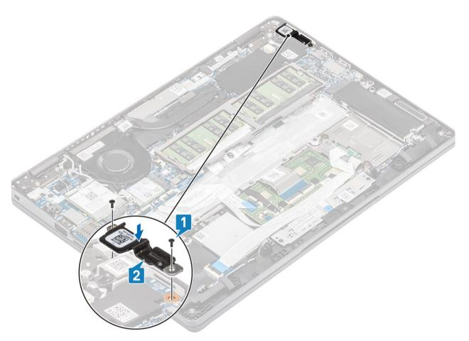
3 Disconnect the DC-in port cable from the connector on the system board and remove the DC-in port from the computer [1, 2].
