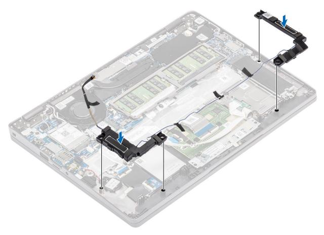
2 Route the speaker cable through the routing guides.
