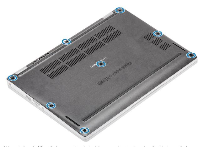
Using a plastic scribe [1], pry the base cover from the top-left corner and continue to work on the sides to open the base cover [2].
