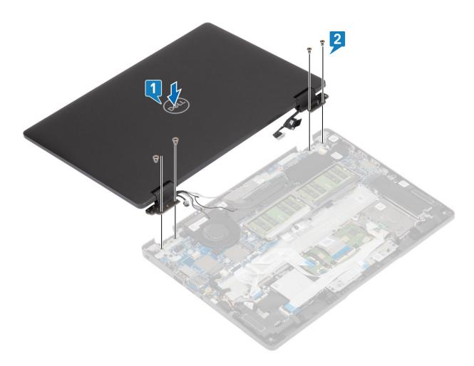
3 Seat the system chassis on the display assembly.
