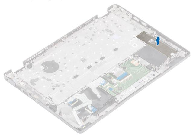
2 Lift the latch and disconnect the backlit cable and the keyboard cable from the connectors on the touchpad.
