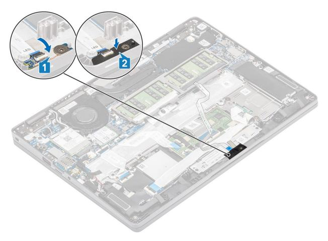
Connect the LED board cable to the connector on the system board and route the LED board cable [1, 2].
