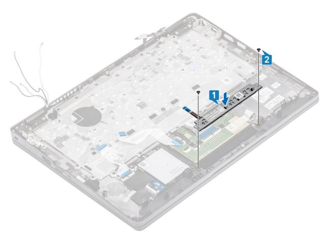
3 Connect the touchpad button board cable to the connector on the touchpad board.
