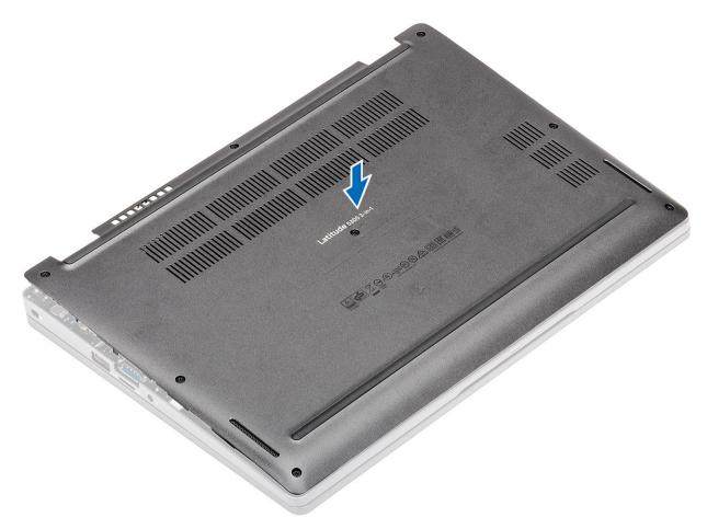
2 Press the edges and sides of the base cover until it snaps into place.
