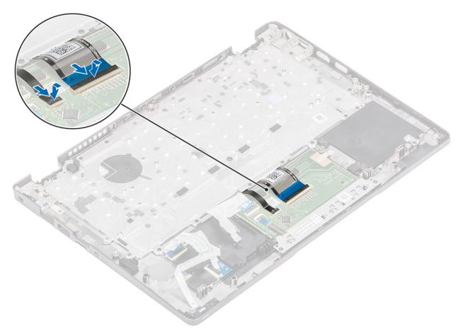
4 Adhere the adhesive tape securing the keyboard and the smartcard board.
