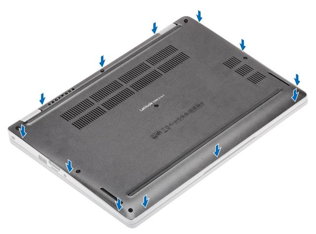
Tighten the eight captive screws to secure the base cover to the computer.
