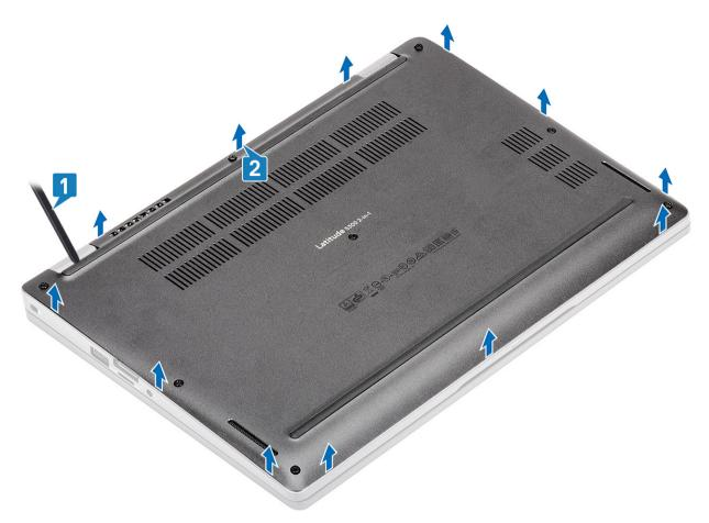
3 Lift and remove the base cover away from the computer.
