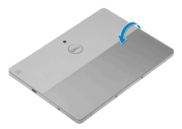
NOTE: Ensure to pry from the docking port and gently moving clockwise to avoid damage to the plastic clips. Use a plastic scribe.
