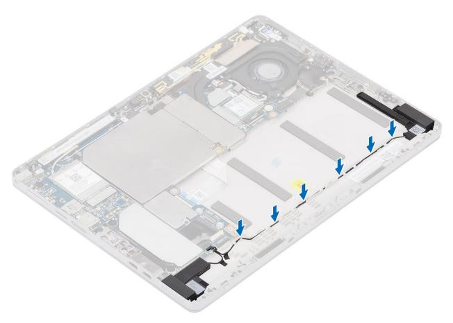
3 Press the speaker and insert it in the slot in the tablet.
