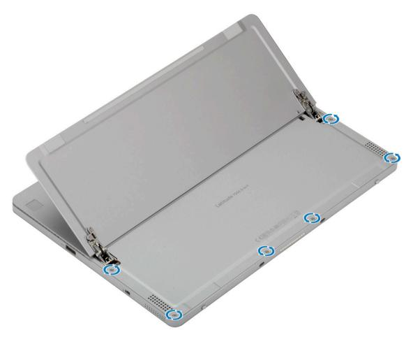
5 Use a plastic scribe [1] to pry the edges [2] of the display panel starting from the bottom side first (near the docking port).
