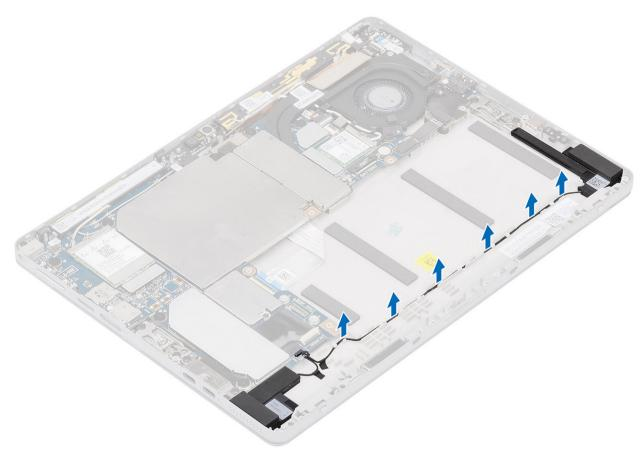
c Using a plastic scribe, peel off and remove both the speakers from the system.
