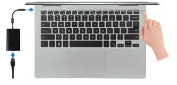
(i) NOTE: To conserve battery power, the battery might enter power saving mode. Connect the power adapter and press the power button to turn on the computer.
