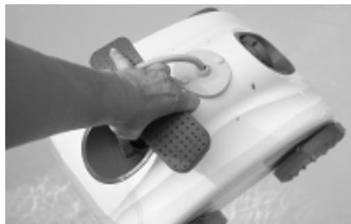
4.2 Place the robot in your pool and wait until it is completely submerged. If necessary, help it to sink manually.
