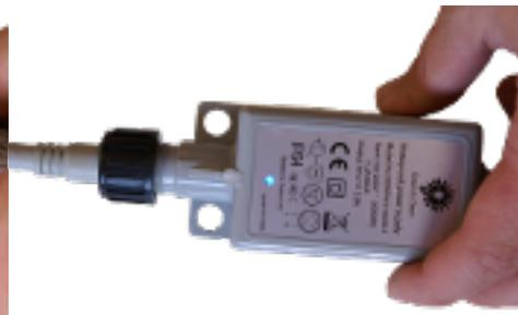
4.5 To Turn off your robot, unplug the transformer. The cleaner will automatically stop after 1 hour of use. To start a new 1 hour cleaning cycle:
