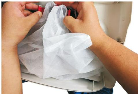
6.2 Pull back the red tabs on one side and completely lift up bag frame on that side.
