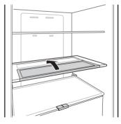
2 Lift the front side of the shelf and shift it under its back side. From this position, both sides of the shelf can be lifted up to free more space. 0
