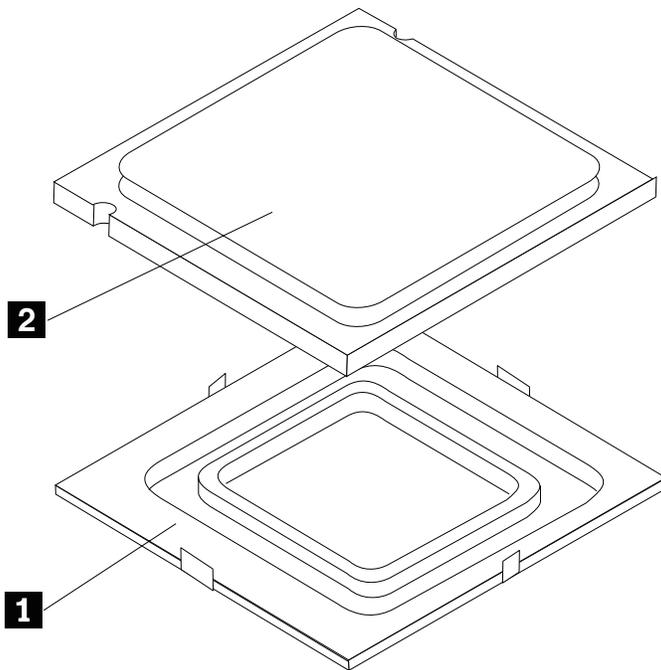
Step 8. Holding the sides of the microprocessor with your fingers, position the microprocessor so that the notches on the microprocessor are aligned with the tabs in the microprocessor socket.
