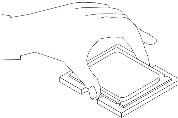
Step 10. To secure the microprocessor in the socket, close the microprocessor retainer and lock it into position with the small handle.
