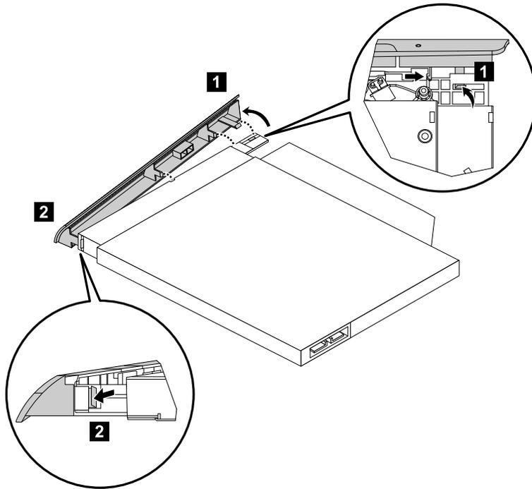
Step 9. To install the new optical drive:
