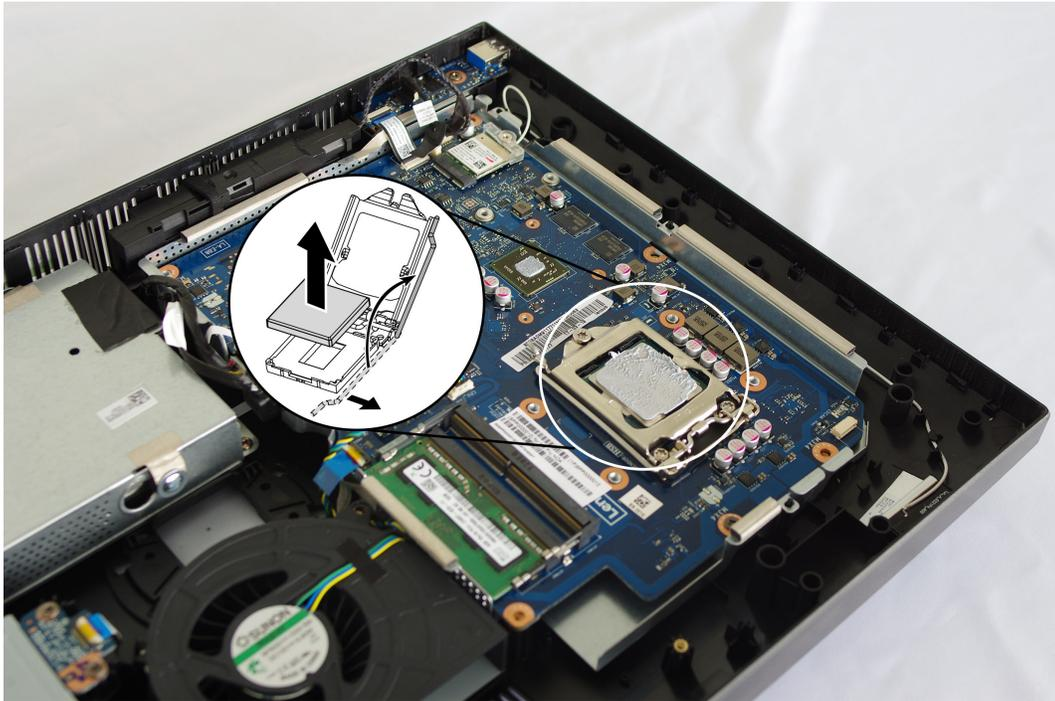
**Attention:** Do not touch the gold contacts on the bottom of the microprocessor. When handling the microprocessor, touch only the sides.
