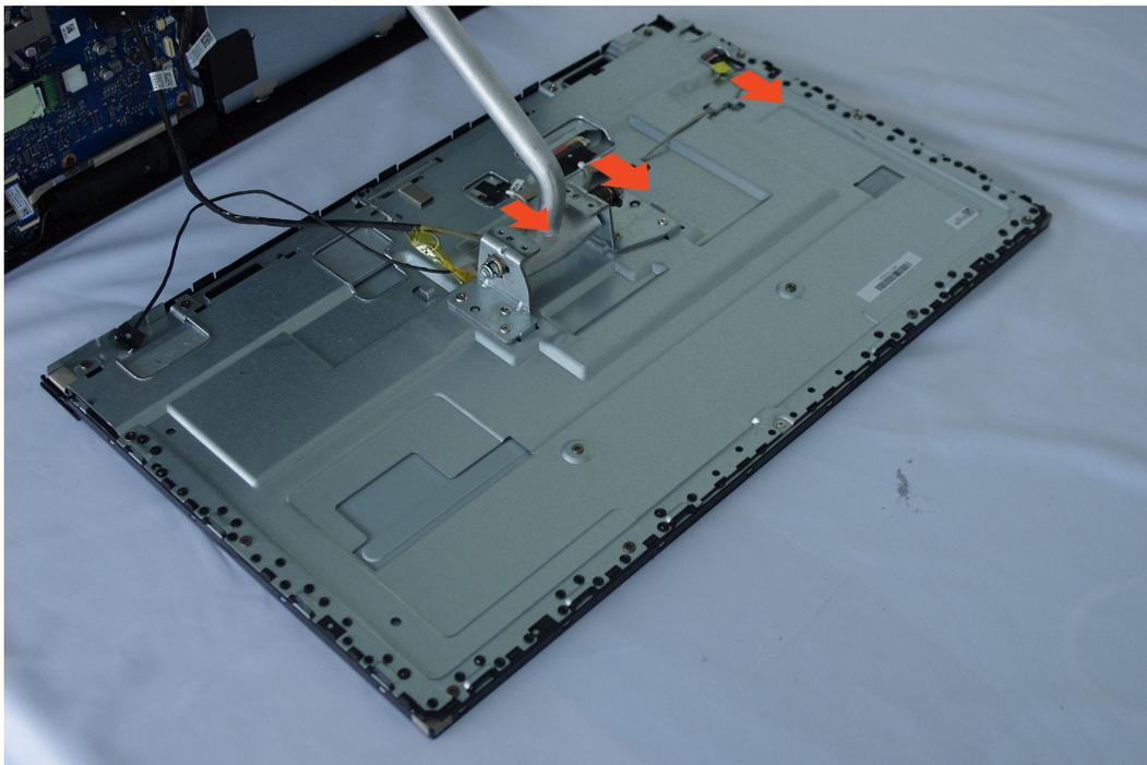
Step 11. To install the new the LCD panel module:
