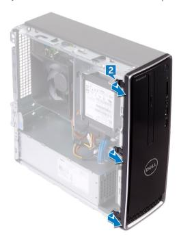
3 Rotate and pull the front bezel away from the computer to release the tabs on the front bezel from the front-panel slots.
