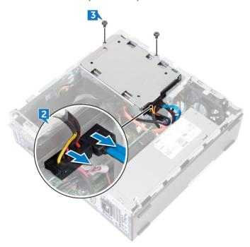
4 Slide the hard-drive assembly toward the inside of the computer and lift it off the drive cage.
