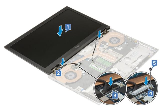
f Align the display hinge caps and replace the 4 (M2.5x4.0) screws to secure the display hinge caps to the system [1, 2].
