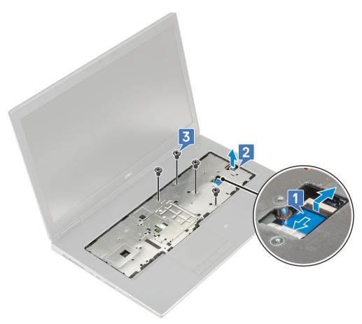
e Push the hole at the bottom of the system to release the palmrest from the bottom chassis.
