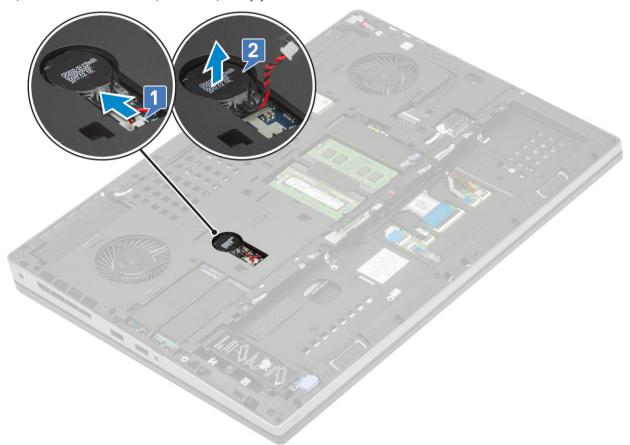
CAUTION: Disconnecting coin cell battery may reset BIOS settings, time and date within System Settings, cause BitLocker or other security resets.
