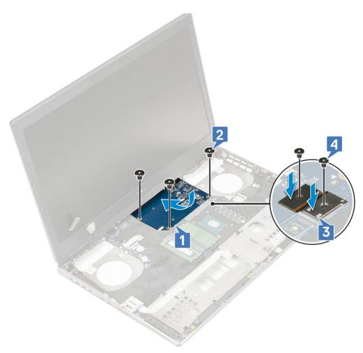
NOTE: The above procedures are for UMA graphics card. Systems shipped with UMA GPU card do not have GPU power cable. However, for discrete models shipped with either a 128 MB or 256 MB VRAM GPU card, you need to connect the GPU power cable after installing the GPU card.
