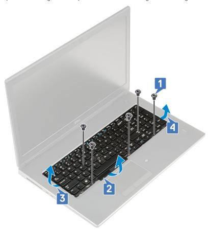
g Slide and remove the keyboard from the system.
