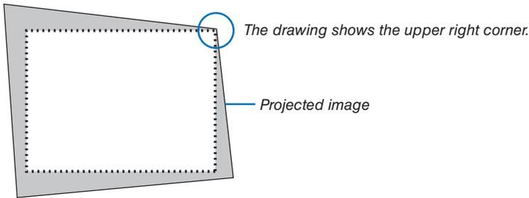
2. Pick up any one of the corners and align the corner of the image with a corner of the screen.
