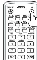
The POWER indicator lit in green will start to blink in blue. After that, the image will be projected onto the screen.
