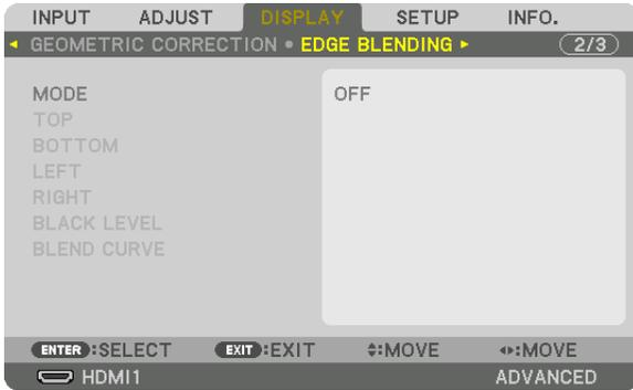
This adjusts the edges (boundaries) of the projection screen when projecting high resolution videos using a combination of several projectors in the up, down, left and right positions.
