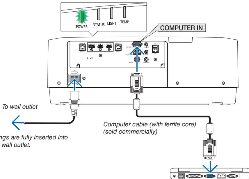
Make sure that the prongs are fully inserted into both the AC IN and the wall outlet.
