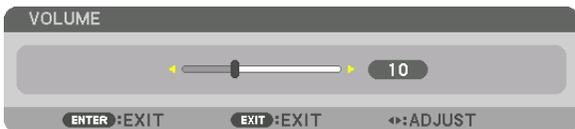
**TIP:** When no menus appear, the ◀ and ▶ buttons on the projector cabinet work as a volume control.
