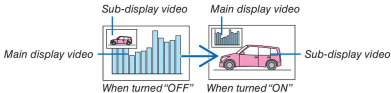
The signal output from the **HDBaseT OUT/Ethernet** terminal does not change even if the display positions are switched.
