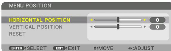
5. Move the cursor either to **[HORIZONTAL POSITION]** or **[VERTICAL POSITION]** by pressing **▼** or **▲** button and then press **◀▶** button to shift the On-Screen Menu.
