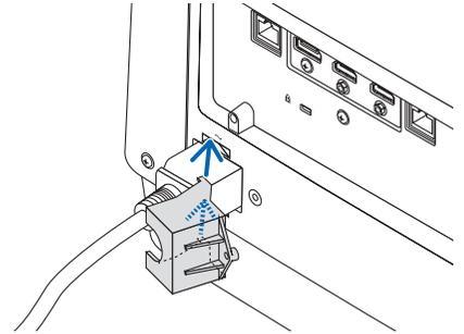
2. **Fasten the screw on the power cord stopper.**
