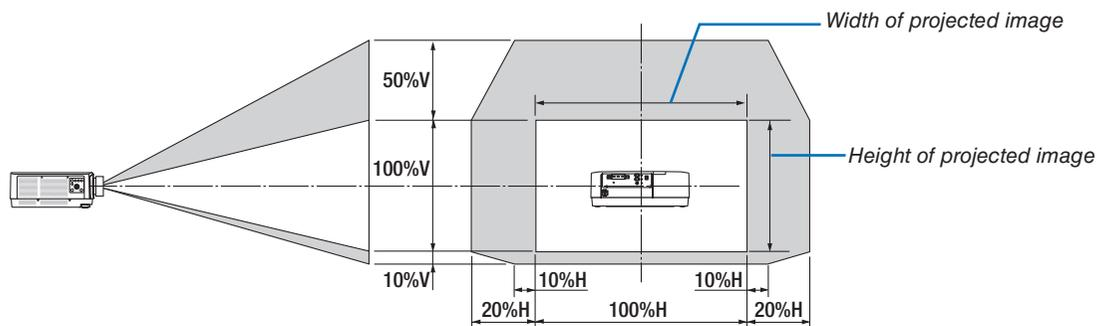
Description of symbols: V indicates vertical (height of the projected image), H indicates horizontal (width of the projected image).
