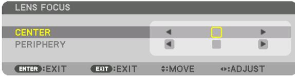
Press ◀▶ buttons to adjust focus. In another way, press and hold the CTL button and then press VOL./FOCUS +/- button on the remote control.
