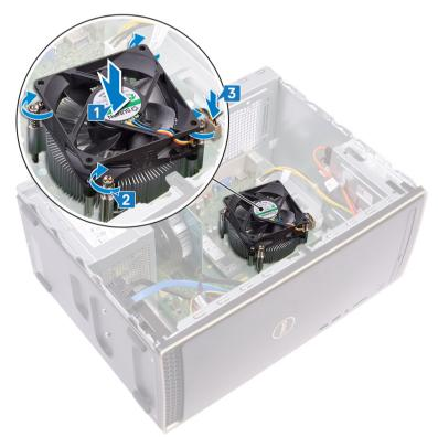
4 Place the fan shroud on the processor fan and heat-sink assembly. Then press down on the fan shroud and snap it into place.
