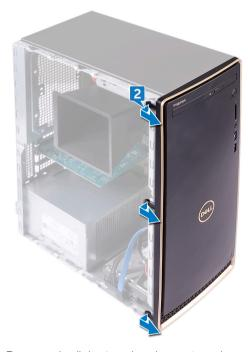
3 Rotate and pull the front bezel away from the computer to release the tabs on the front bezel from the slots on the chassis.
