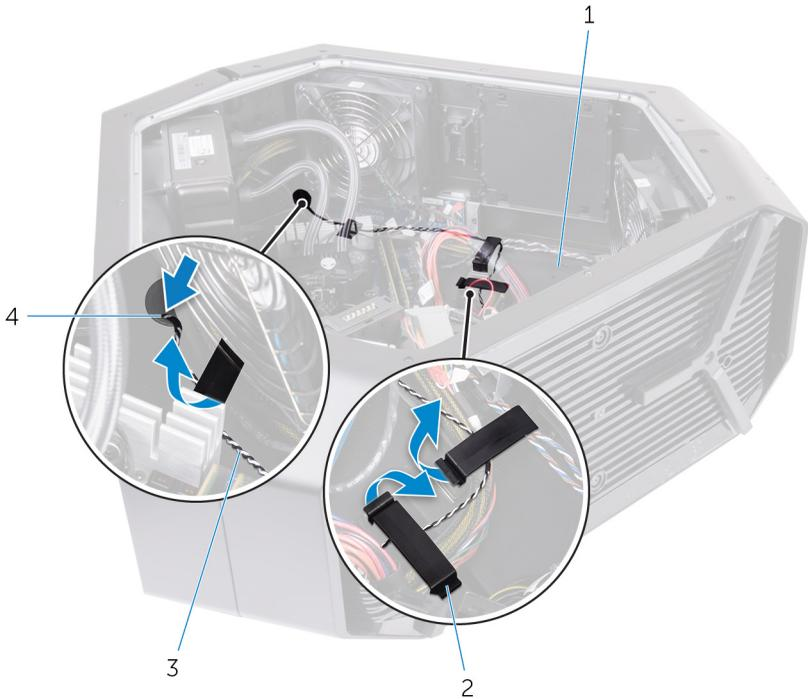
**Figure 65. Removing the rear I/O accessibility lighting cable**
