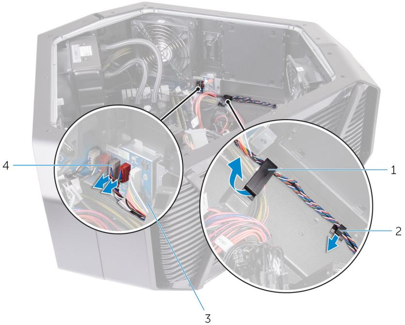
**Figure 76. Removing the bottom tron-lighting cables**
