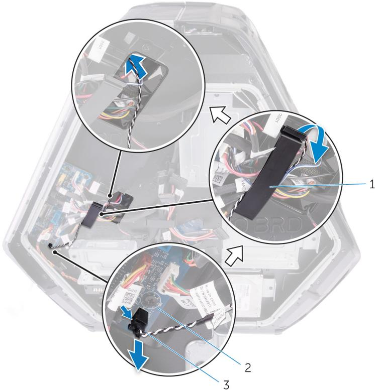
**Figure 64. Removing the rear I/O accessibility lighting cable**
