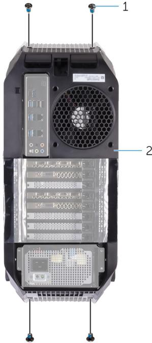
**Figure 67. Removing the rear bezel**
