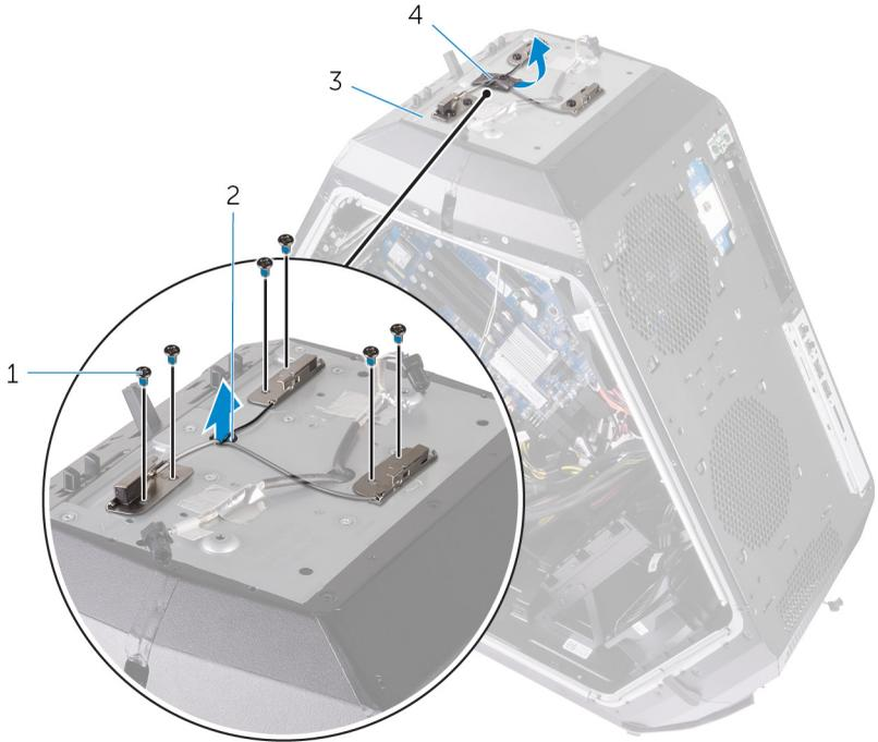
**Figure 81. Removing the antenna cables**
