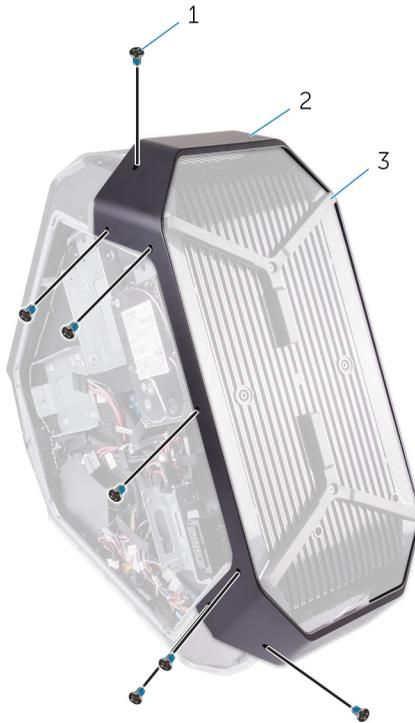
**Figure 56. Removing the screws**
