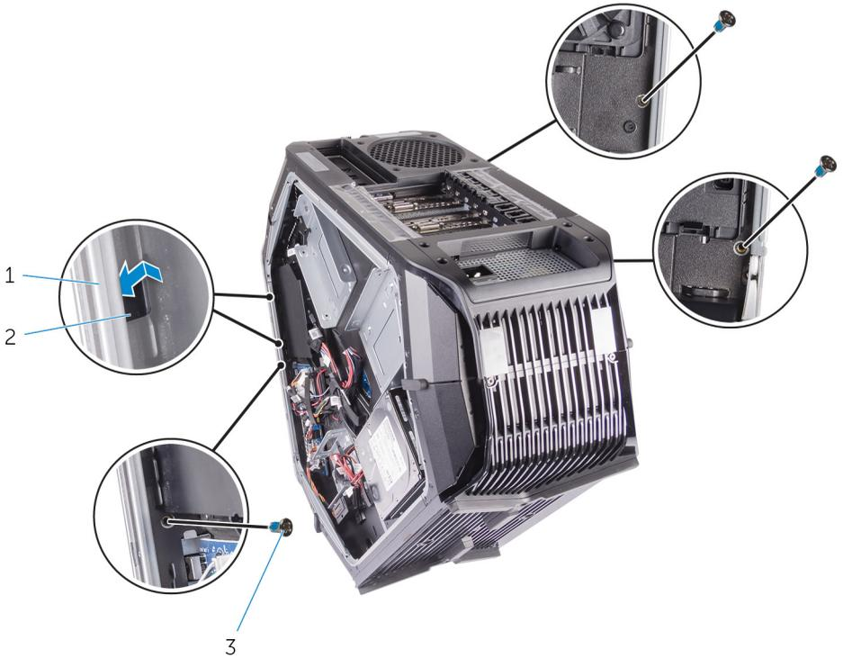
**Figure 59. Removing the screws**
