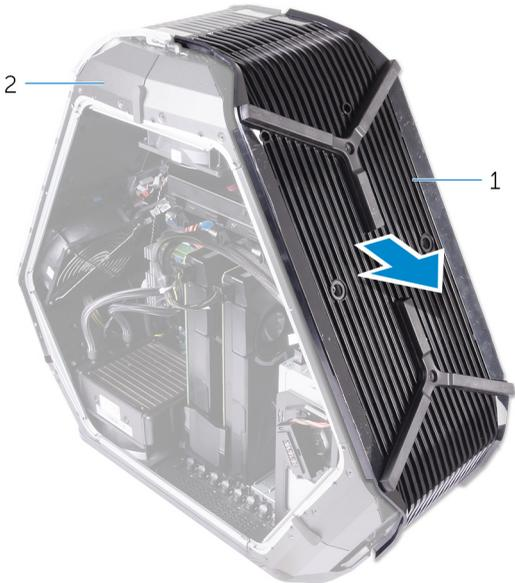
Figure 73. Removing the base panel
