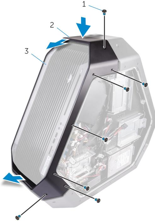
**Figure 55. Removing the front-handle bar**
