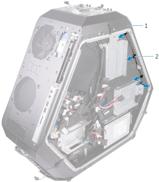
**Figure 79. Removing the antenna cables**
