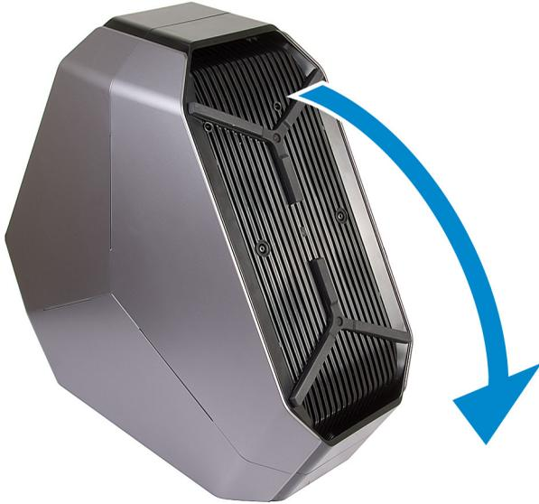
**Figure 7. Tilt the computer to upright position**
