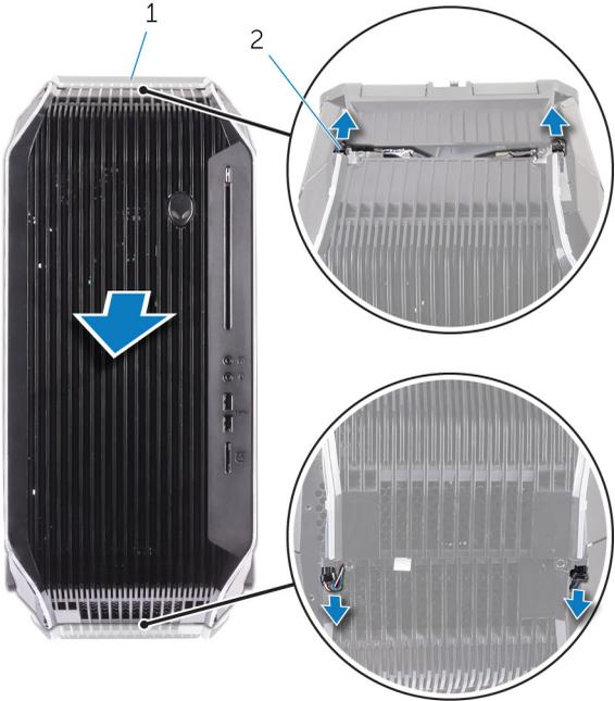
Figure 60. Removing the front bezel
