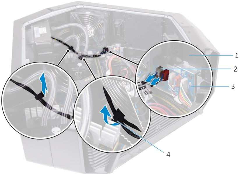
**Figure 74. Removing the top tron-lighting cables**
