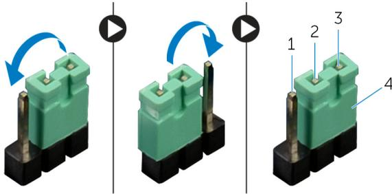
**Figure 83. Clearing CMOS settings**
