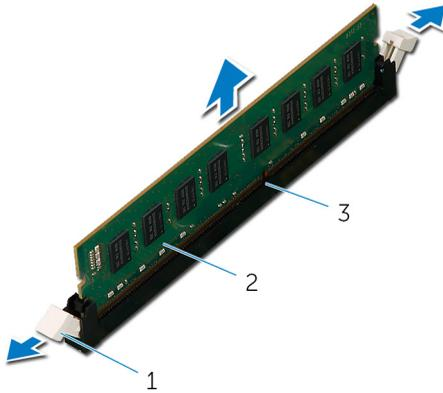
**Figure 24. Removing the memory module**
