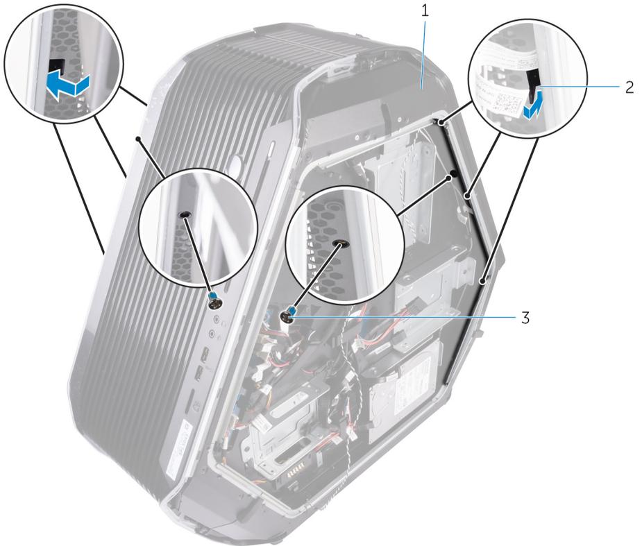
**Figure 68. Removing the rear bezel**
