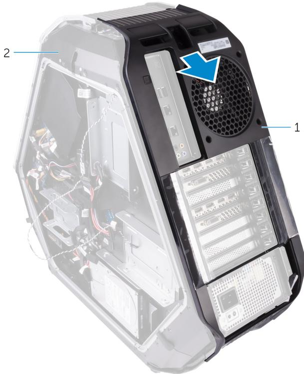
**Figure 69. Removing the rear bezel**
