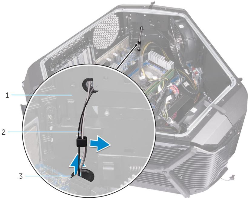
**Figure 80. Removing the antenna cables**
