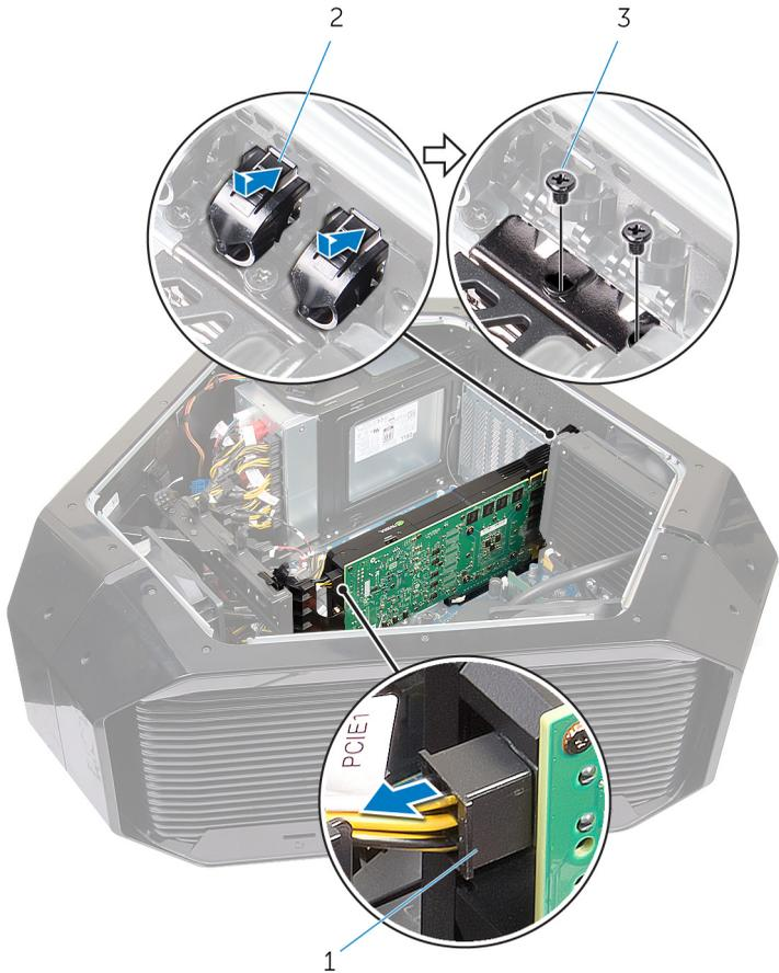
**Figure 31. Removing the Full length graphics card**
