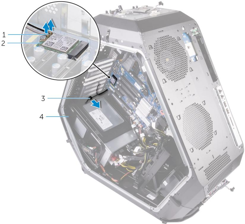
**Figure 78. Removing the antenna cables**
