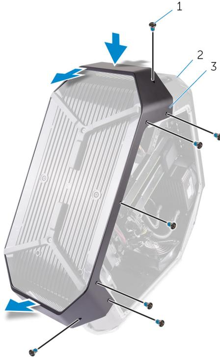
**Figure 57. Removing the bottom-handle bar**
