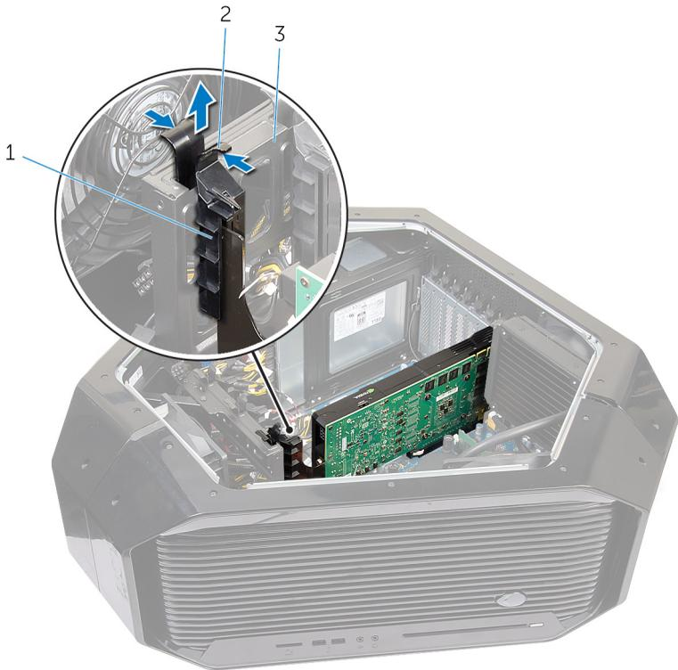
**Figure 30. Removing the Full length graphics card**
