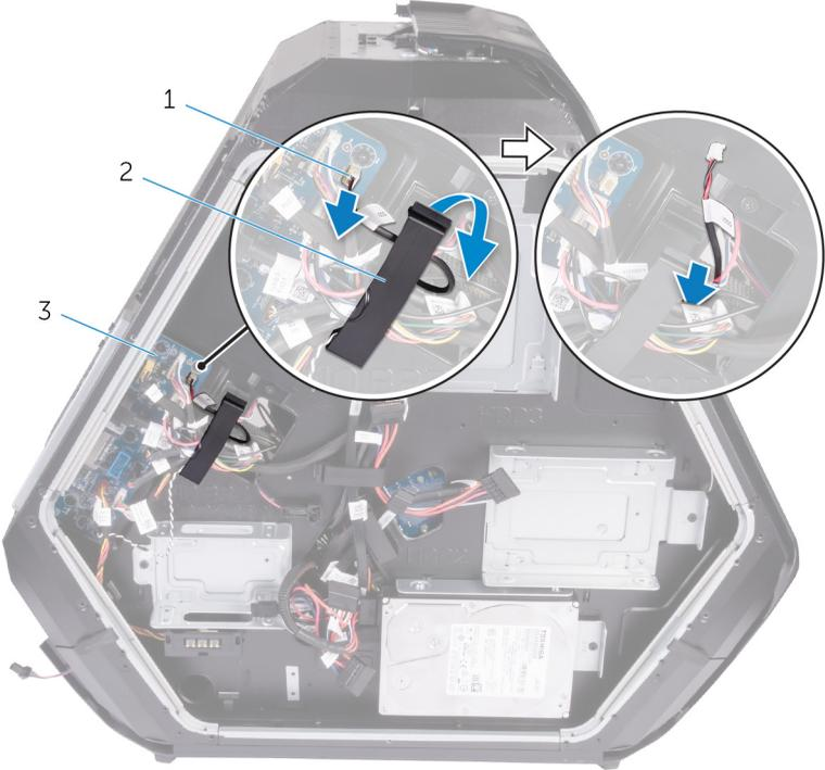
**Figure 61. Removing the optical-drive eject-button board cable**
