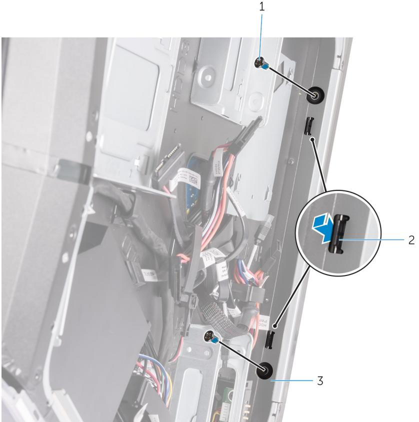
**Figure 72. Removing the base panel**
