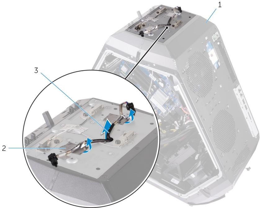
**Figure 75. Removing the top tron-lighting cables**
