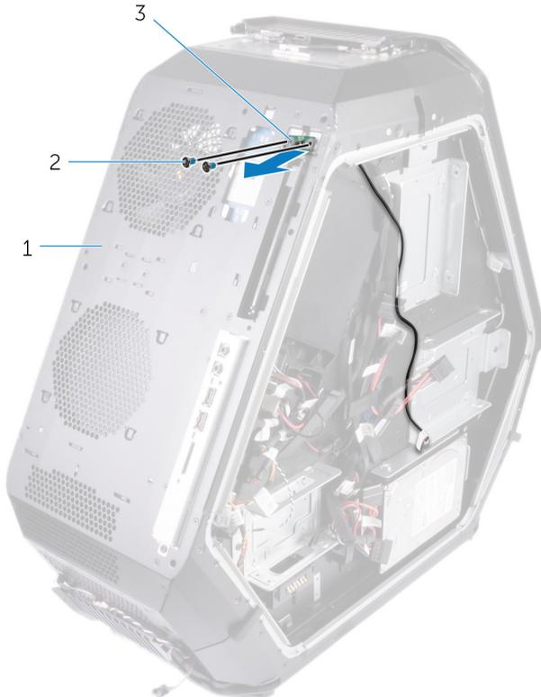
**Figure 63. Removing the optical-drive eject-button board**
