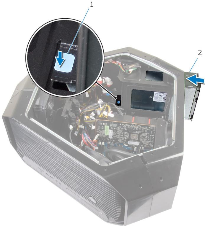
**Figure 50. Replacing the power-supply unit**
