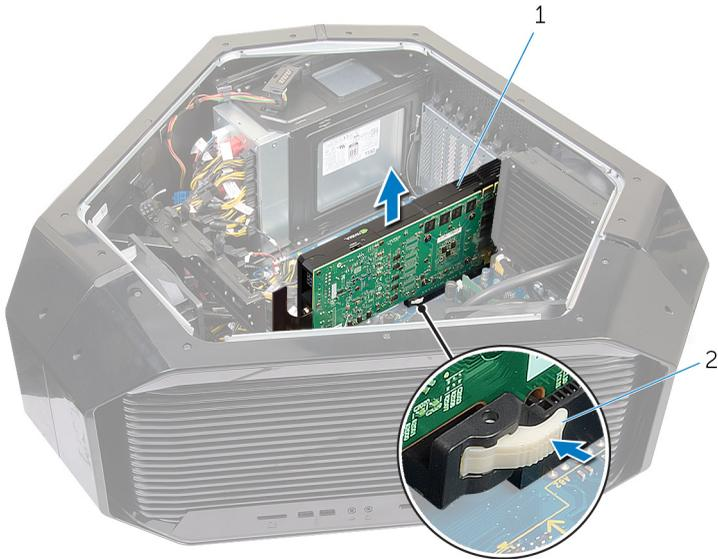
**Figure 32. Removing the Full length graphics card**
