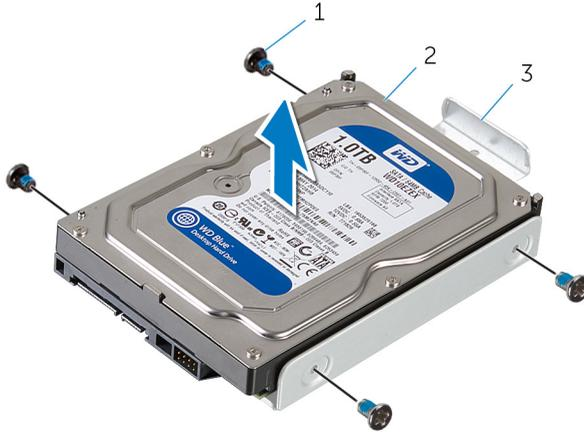
**Figure 12. Removing the hard-drive bracket**
