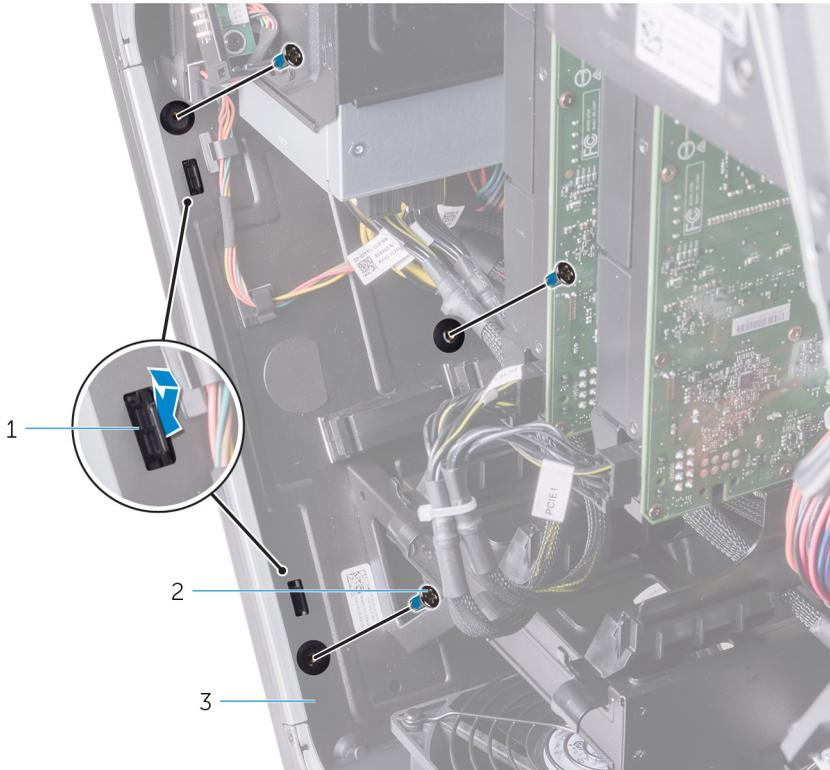
**Figure 71. Removing the base panel**
