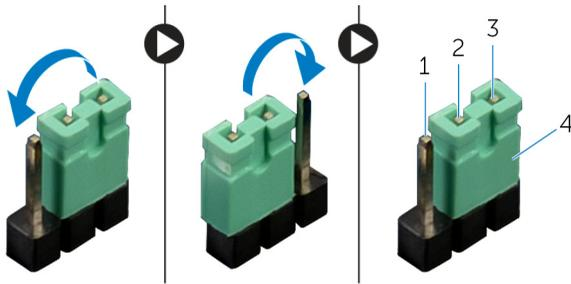
**Figure 82. Clearing forgotten passwords**
