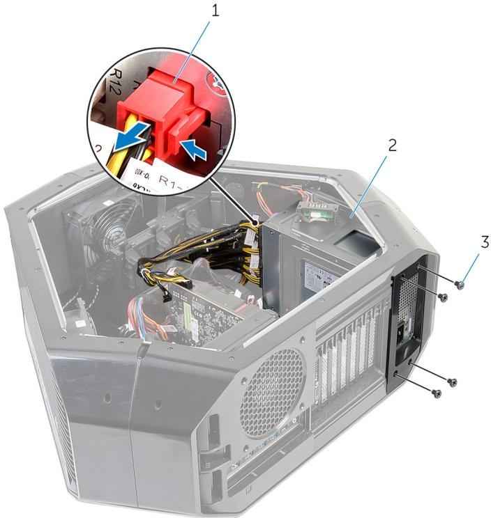
**Figure 47. Removing the power-supply unit**
