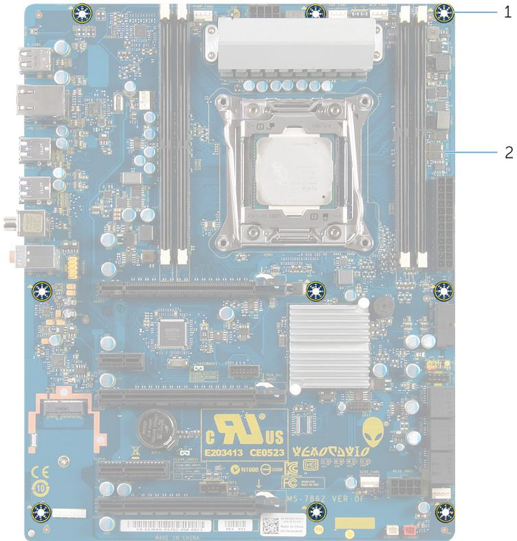
**Figure 51. Removing the system board**
