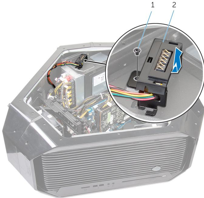
**Figure 18. Image: Left AlienFX connector removal**
