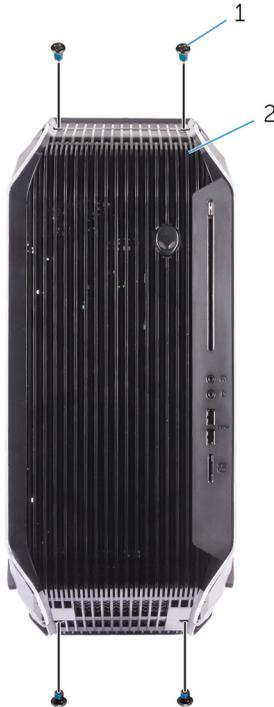
**Figure 58. Removing the screws**
