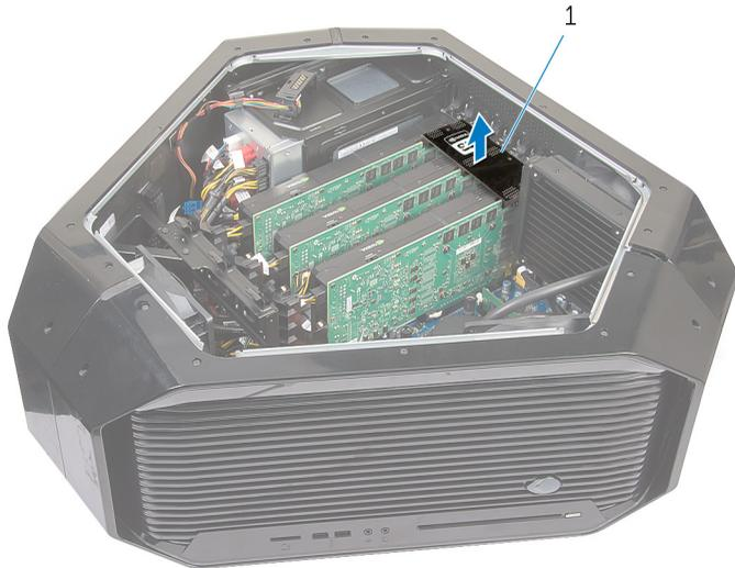
**Figure 27. Removing the graphics bridge**
