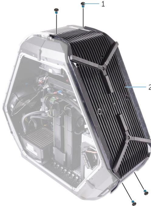
**Figure 70. Removing the base panel**
