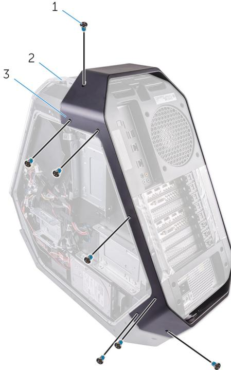
**Figure 52. Removing the screws**
