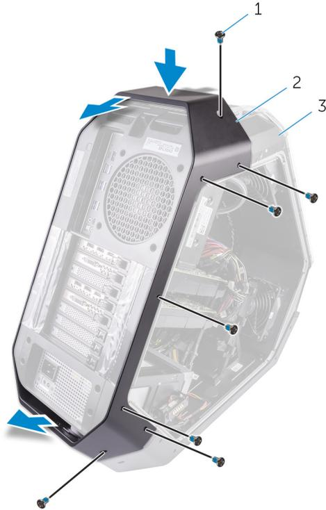
**Figure 53. Removing the rear-handle bar**
