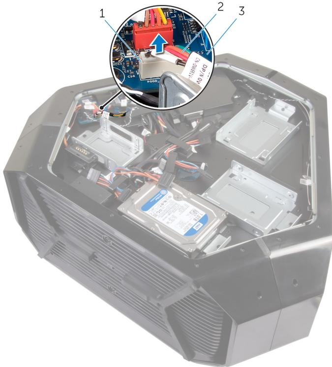
**Figure 17. Image: Left AlienFX connector removal**
