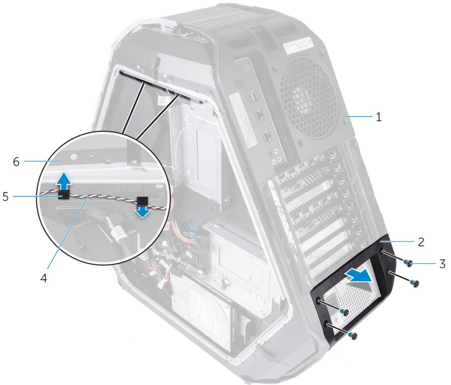
**Figure 66. Removing the rear I/O accessibility lighting cable**
