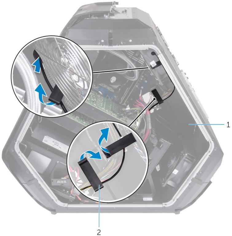
**Figure 62. Removing the optical-drive eject-button board cable**
