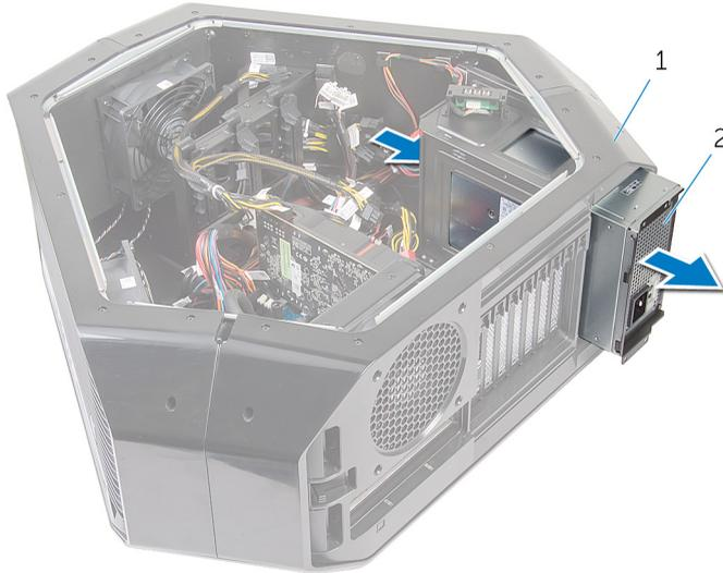
**Figure 49. Removing the power-supply unit**
