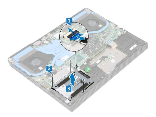
Disconnect the interposer from the hard-drive assembly.
