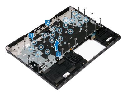
4 Lift the keyboard, along with its cable, off the palm-rest assembly.
