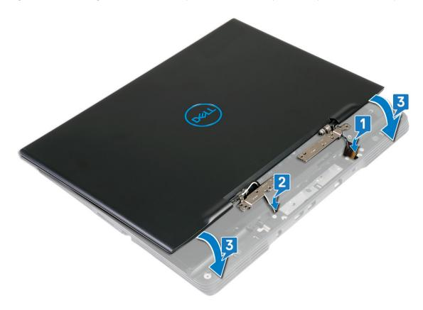
4 Replace the eight screws (M2x4) that secure the left and right hinges to the palm-rest assembly.
