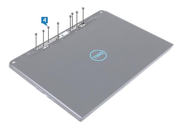
Align the hinge cover with the slots on the palm-rest assembly and press to secure the hinge cover.
