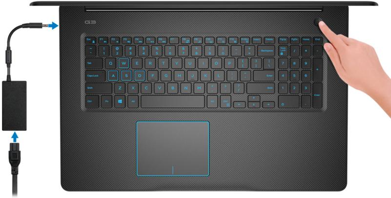
**NOTE:** To conserve battery power, the battery might enter power saving mode. Connect the power adapter and press the power button to turn on the computer.
