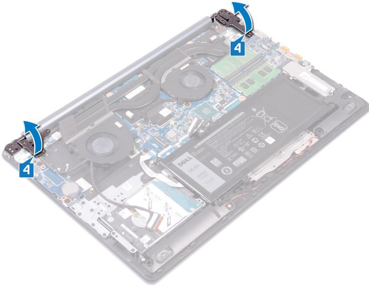
5 Lift the palm rest and keyboard assembly at an angle.
