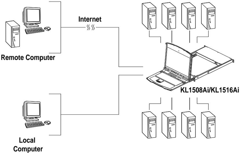
By daisy chaining up to 15 additional switches, as many as 256 computers can be controlled from the original KVM console. An auto-sensing function recognizes the position of each station on the chain, eliminating the need to manually set the position, and a two digit seven-segment LED display on the keyboard module showing each station's position for easy identification.
