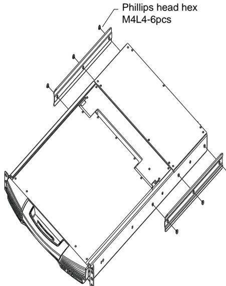
2. Attach the left and right *easy-installation* mounting rails to the inside of the rack. The flange that supports the switch will be to the inside.
