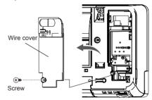
(3) Remove the tapping screw and while minding the cable clamp hook, remove the cable clamp
