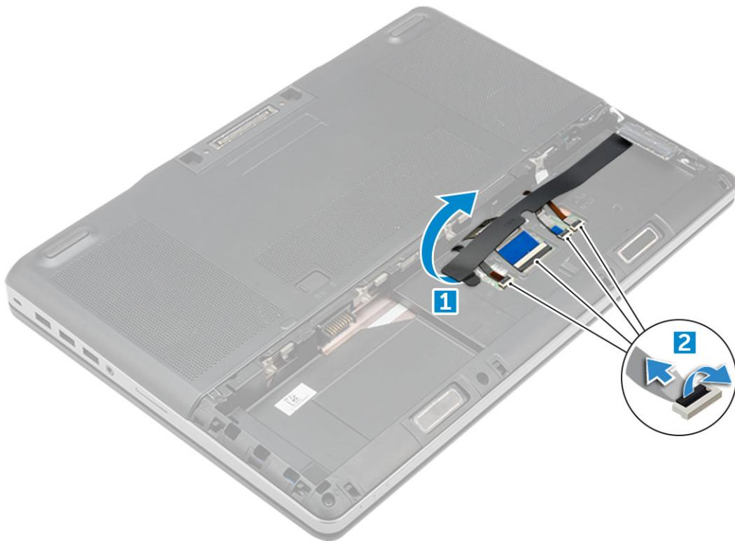
a Peel the tape to access the keyboard cable [1].
