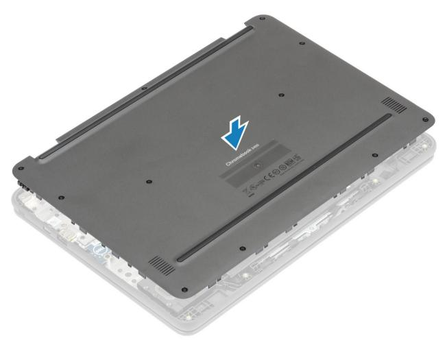
2 Tighten the 11 captive screws to secure the base cover to the computer.
