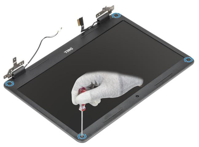
Use a plastic scribe to carefully pry open the upper right or upper left corner of the outside edge of the display bezel and continue to pry open the outside edge of the top side of the display bezel and then pry open the outside edge of the left and right sides of the display bezel [1, 2, 3].
