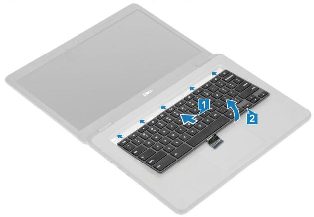
2 Carefully insert the keyboard cable through the gap on the palm rest and place the keyboard trim to its place [1, 2].
