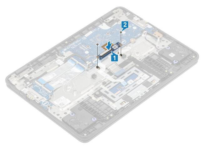
3 Connect the keyboard cable and keyboard interposer board cable to the connectors on the interposer board and system board [1, 2].
