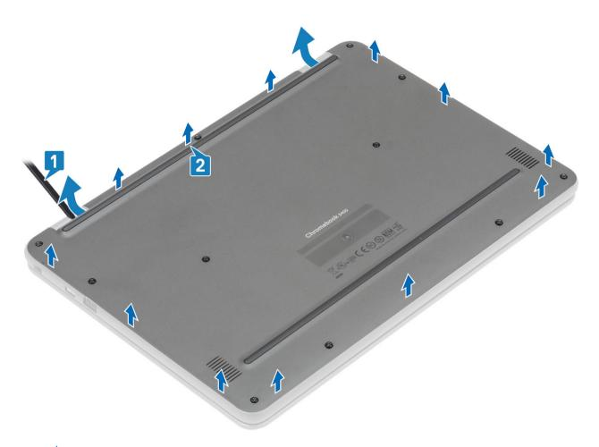
NOTE: While removing the base cover, on-site technicians must take care to remove the base cover carefully. There are prying recess points next to the left and right hinges which ease the disassembly procedure. With the help of a plastic scribe, pry open from the top left side of the base cover, continue working your way around the left and right side of the base cover, then remove the base cover from the system.
