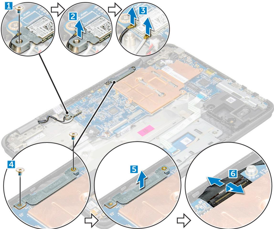
4 Disconnect the sensor cable, and turn over the computer [1, 2]
