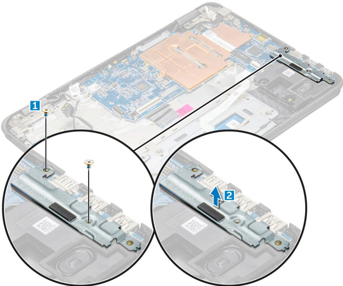
5 To remove the metal bracket (WLAN and display cable):
