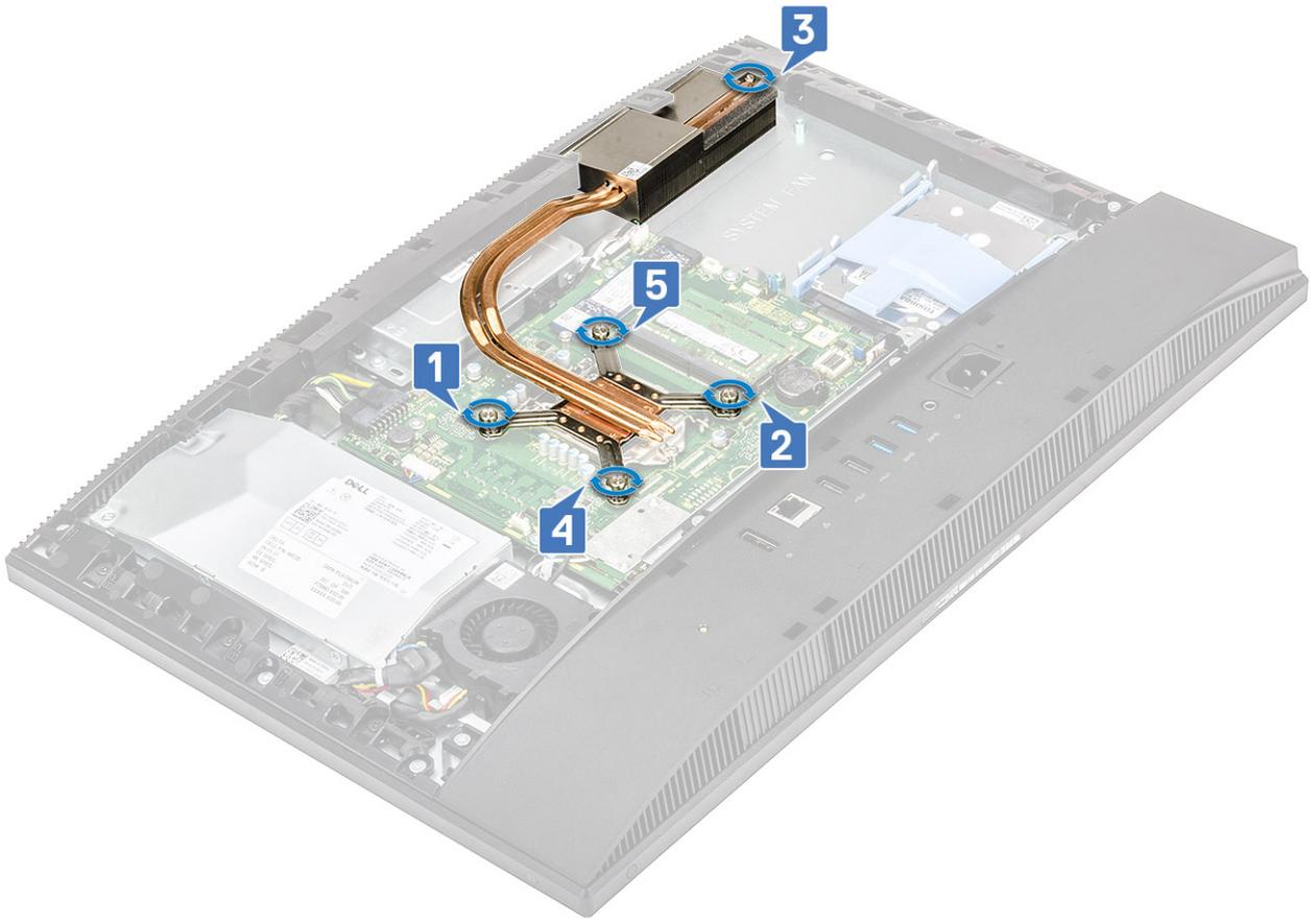
4. Lift the heat sink off the system board and display assembly base .
