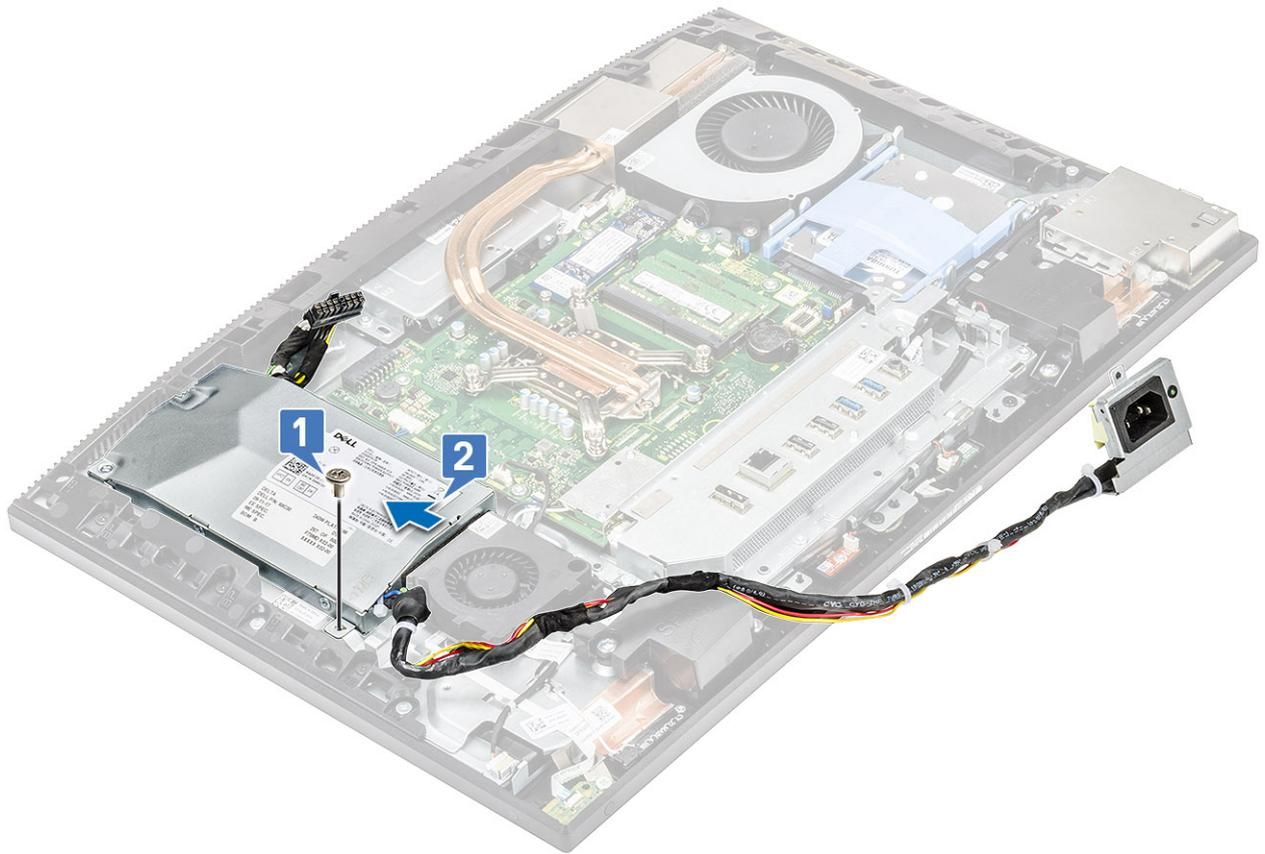
b) Slide the PSU, and lift it away from the chassis .
