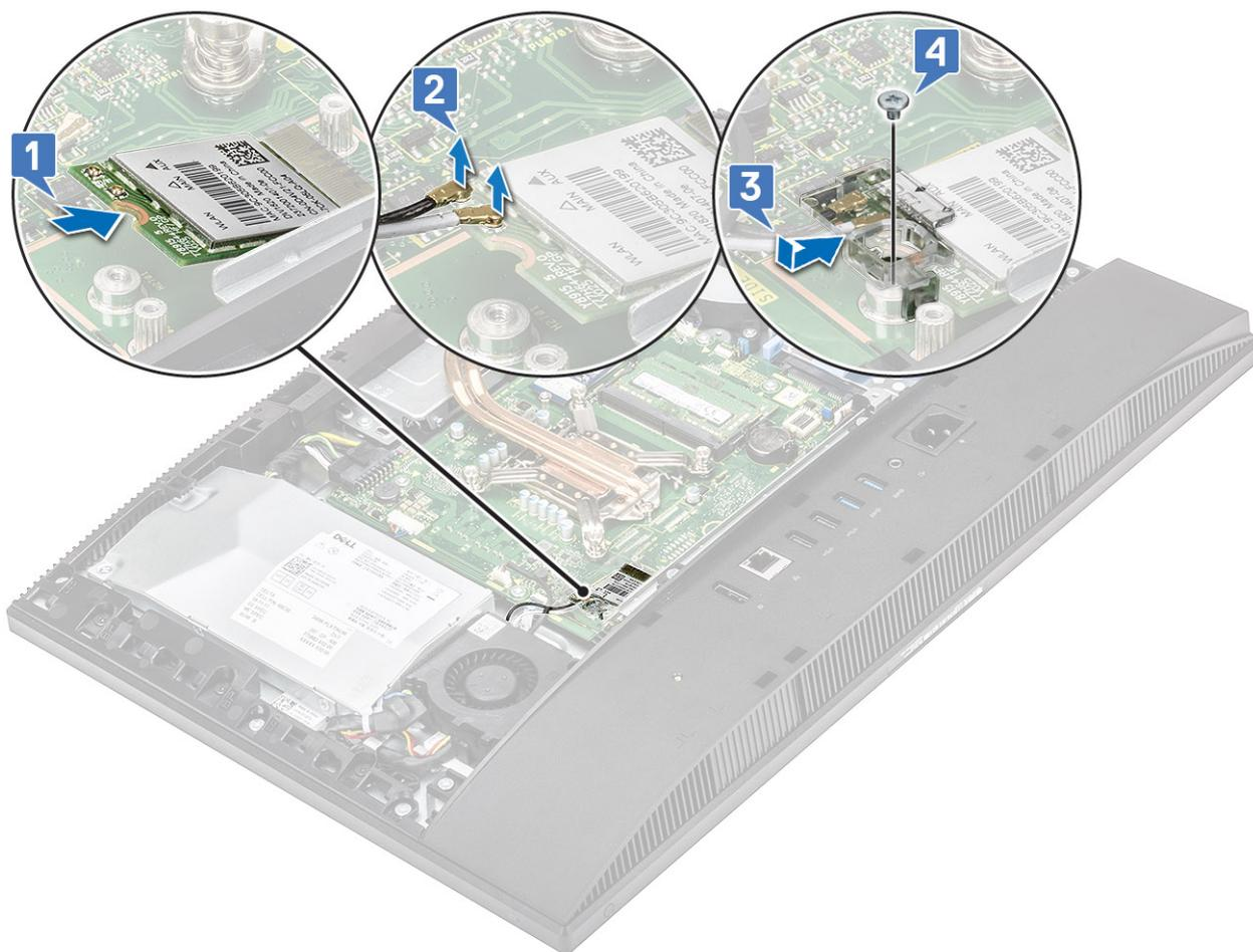
2. To install the WLAN card shield:
