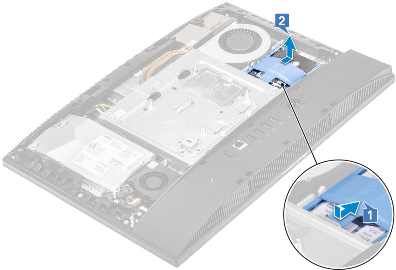
4. To remove the hard drive bracket:
