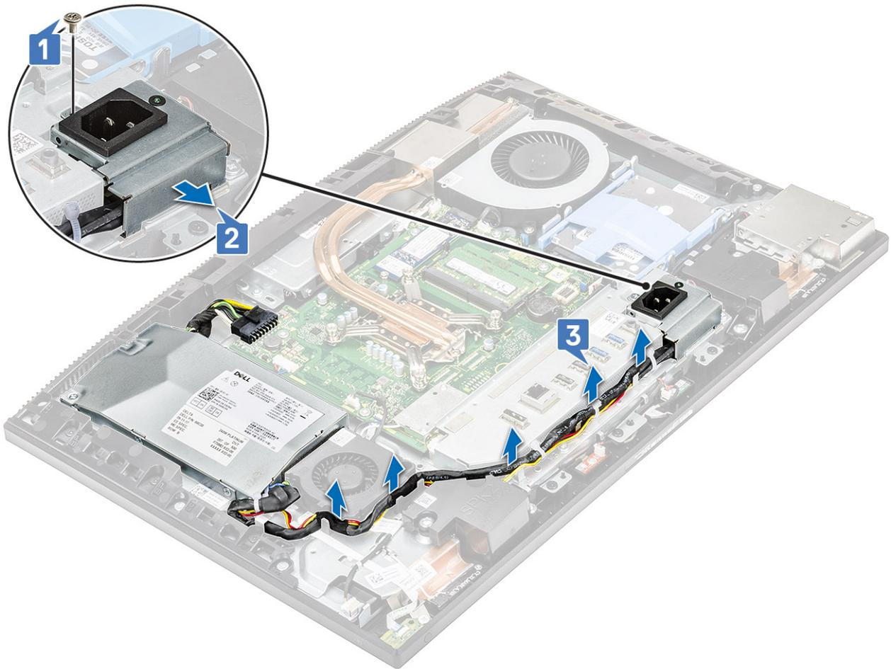
5. To remove the Input and Output (I/O) bracket:
