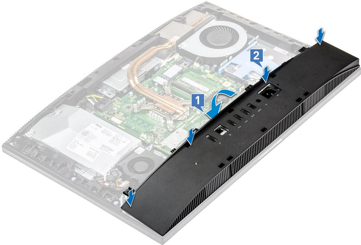
3. Replace the four screws (M3x5) that secure the base cover to the display assembly base.
