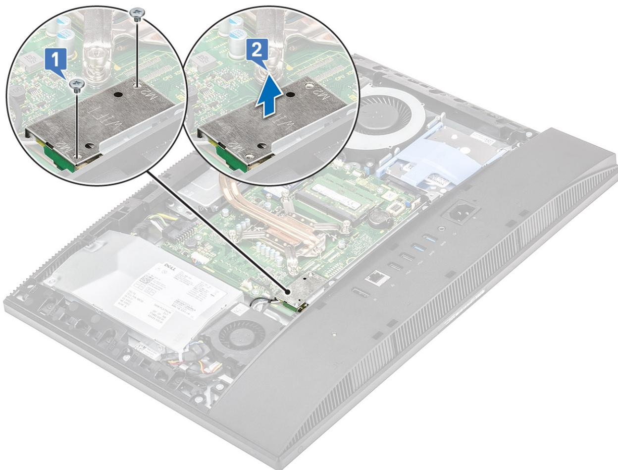
**4.** To remove the WLAN card:
