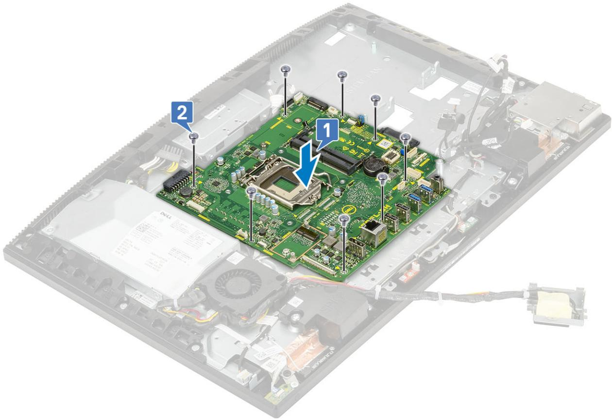
**3.** Connect the following cables to the system board:
