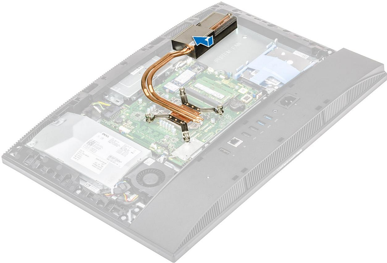
2. Tighten the five captive screws in a sequential order [1,2,3,4,5] to secure the heat sink to the system board and display assembly base..
