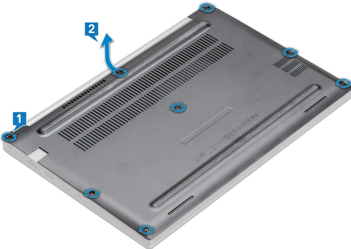
**CAUTION:** Exercise caution when loosening the screws. Angle the screwdriver to match the head of the screw (front corners on the laptop base cover) to avoid a possible stripped screw head.
