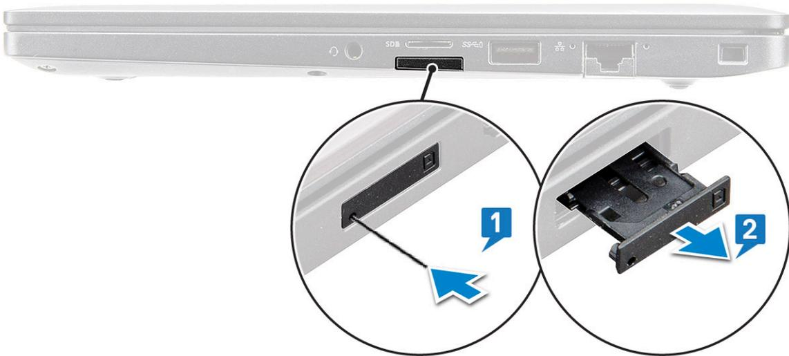
**NOTE:** For Latitude 7390 , the SD memory card must be removed before replacing any system components. Failure to remove the SD memory card before the disassembly of other components may result in damage to the system
