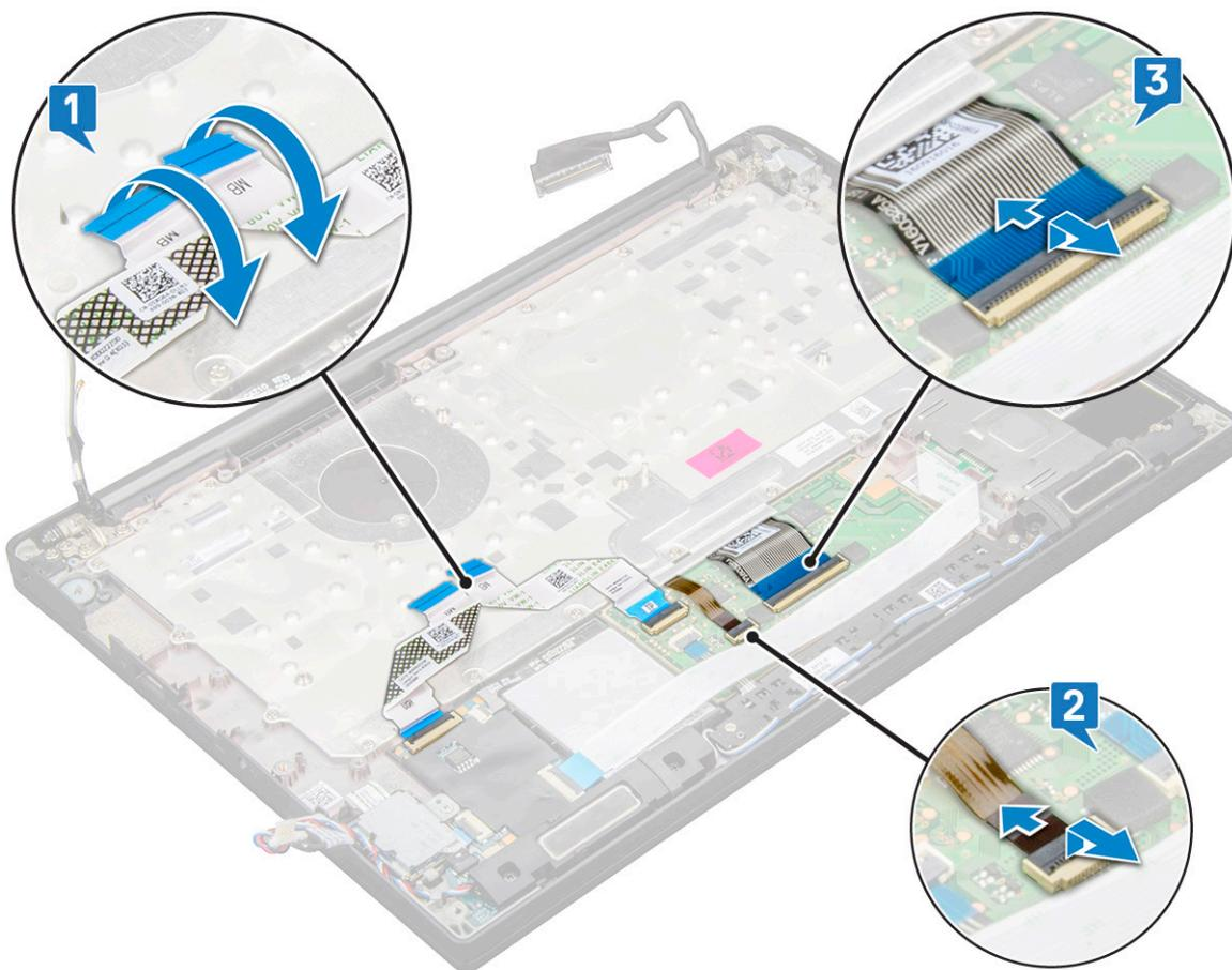
4 To remove the keyboard assembly:
