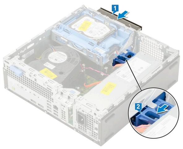
**3.** Lift the hard drive and optical module [1], connect the optical drive data cable and power cable to the connectors on the optical drive [2, 3].
