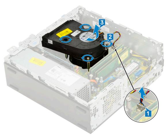
(i) NOTE: Loosen the screws in a sequential order (1,2,3,4) as mentioned on the system board.
