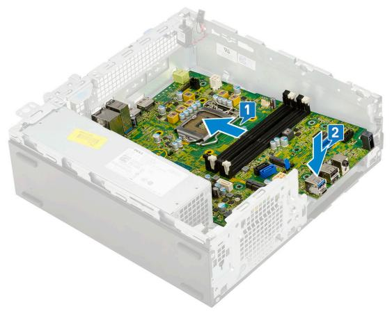
**3.** Replace the standoff single (#6-32) screw, the single screw used as a mounting point for M.2 SSD drive and the 5 screws that secure the system board to the system [1, 2, 3][1,2].
