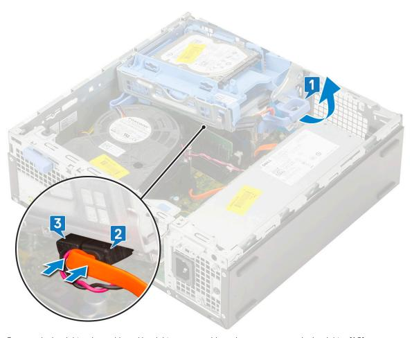
4. Connect the hard drive data cable and hard drive power cable to the connectors on the hard drive [1,2].
