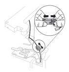
4 Unscrew the groud wire 1. Rotate the hinge lever counterclockwise. Lift the top hinge free of the hinge lever latch.
