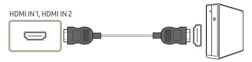
When connecting an HDMI cable, use the cable that came with the components of the monitor. If you use an HDMI cable other than provided by Samsung, the image quality may be degraded.
