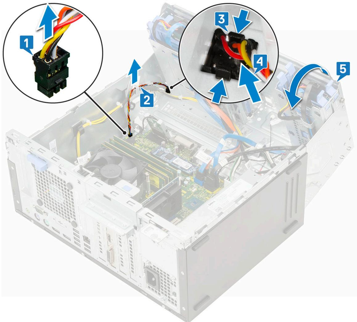
5 Pull the power switch out from the computer.
