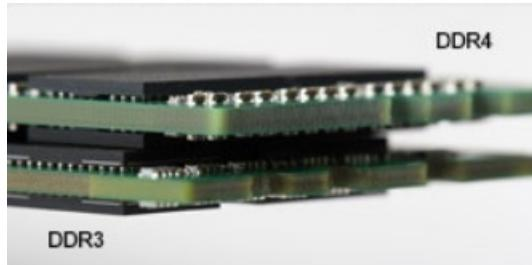
**Figure 2. Thickness difference**
