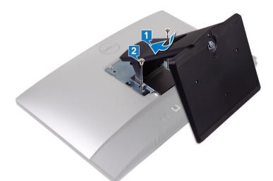
3 Snap the tabs on the stand cover into the slots on the back cover.
