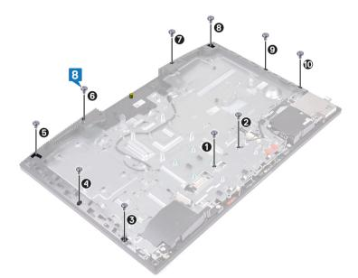
9 Remove the jig screw from the display panel.
