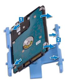
3 Place the hard-drive assembly into its slot and slide to lock the hard-drive assembly to the display-assembly base.
