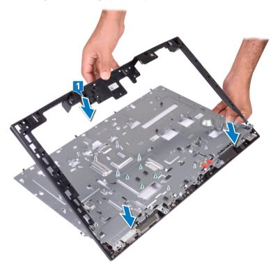
2 Replace the 17 screws (M3x5) that secure the middle frame to the display-assembly base.
