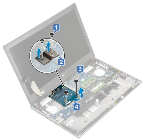
NOTE: The above procedures are for UMA graphics card. Systems shipped with UMA GPU card do not have GPU power cable. However, for discrete models shipped with either a 128 MB or 256 MB VRAM GPU card, you need to disconnect the GPU power cable before removing the GPU card.
