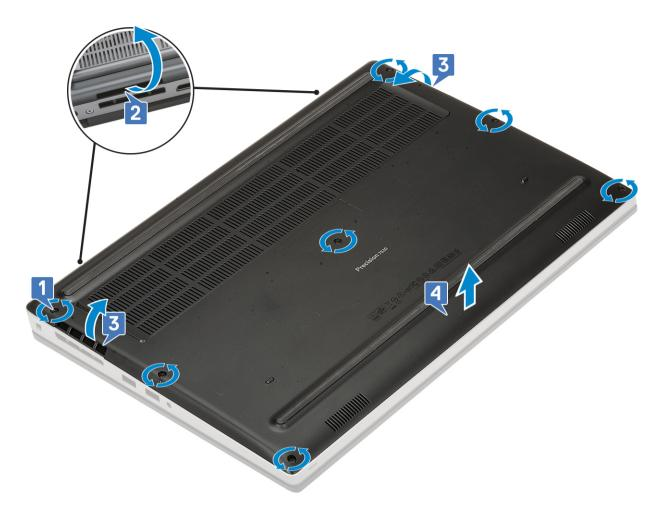
NOTE: While pry open the base cover make sure to use hands or plastic scribe—do not use any other sharp objects as it may damage the chassis
