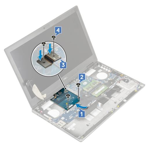
NOTE: The above procedures are for UMA graphics card. Systems shipped with UMA GPU card do not have GPU power cable. However, for discrete models shipped with either a 128 MB or 256 MB VRAM GPU card, you need to connect the GPU power cable after installing the GPU card.
