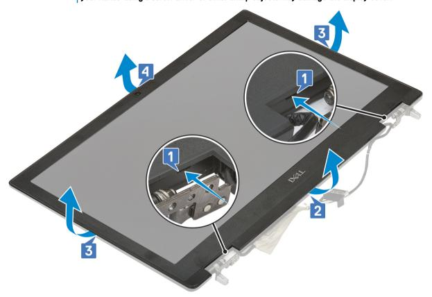
NOTE: The display bezel shipped with a non-touch display is a disposable part and should be replaced with a new display bezel anytime it is removed from the system.
