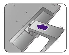
Tighten the screw(s) that fixes the stand to the monitor.
