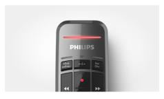
The record LED makes it easy to monitor the recording status without looking at the computer screen. The indicator light glows in red in overwrite mode or green in insert mode while recording preventing you from dictating without actually recording or accidentally overwriting a file.
