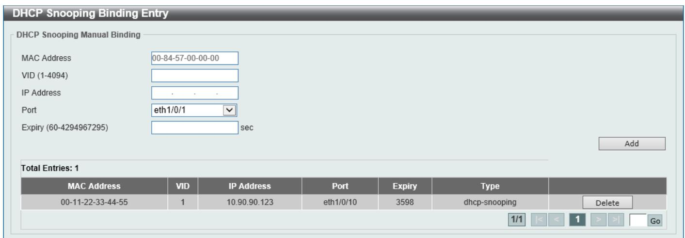
Figure 9-36 DHCP Snooping Binding Entry Window
