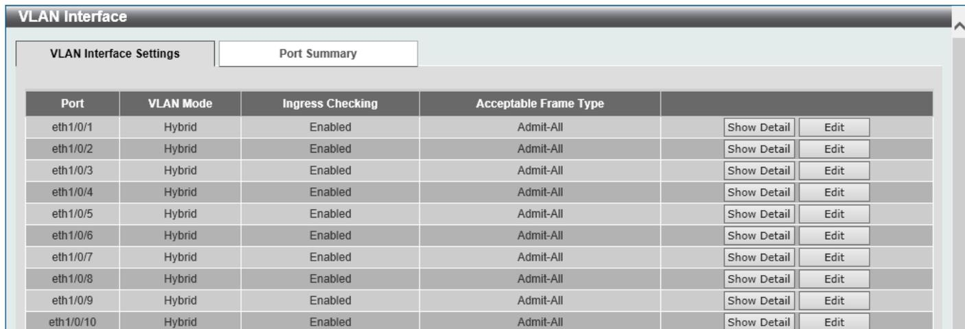
The screenshot shows the 'VLAN Interface' window with two tabs: 'VLAN Interface Settings' (selected) and 'Port Summary'. Below the tabs is a table with columns: Port, VLAN Mode, Ingress Checking, Acceptable Frame Type, Show Detail, and Edit. The table lists 10 ports (eth1/0/1 to eth1/0/10) with Hybrid VLAN Mode, Enabled Ingress Checking, and Admit-All Acceptable Frame Type.
