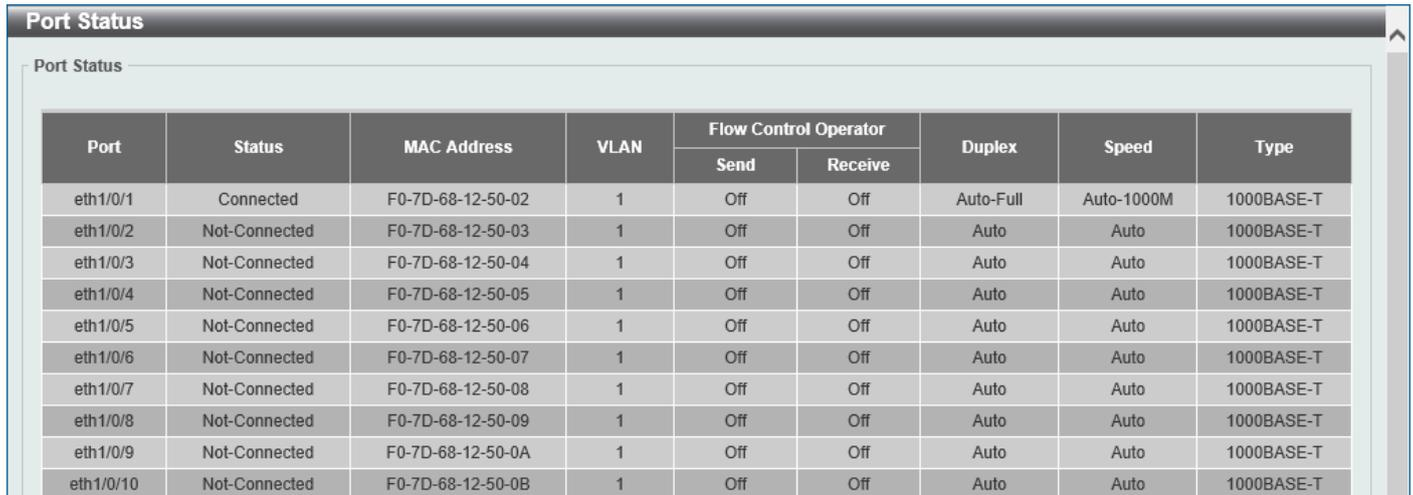
The screenshot shows the 'Port Status' window with a table listing 10 ports (eth1/0/1 to eth1/0/10). The table columns are Port, Status, MAC Address, VLAN, Flow Control Operator (Send, Receive), Duplex, Speed, and Type. Port eth1/0/1 is 'Connected', while all other ports are 'Not-Connected'.
