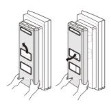
2 Remove the contents of the drawer. Hold the handle of the drawer and gently pull it out completely until it stops. Repeat to remove the second drawer.
