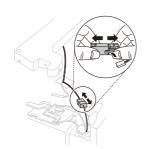
3 Unscrew the groud wire **1**. Rotate the hinge lever counterclockwise. Lift the top hinge free of the hinge lever latch.
