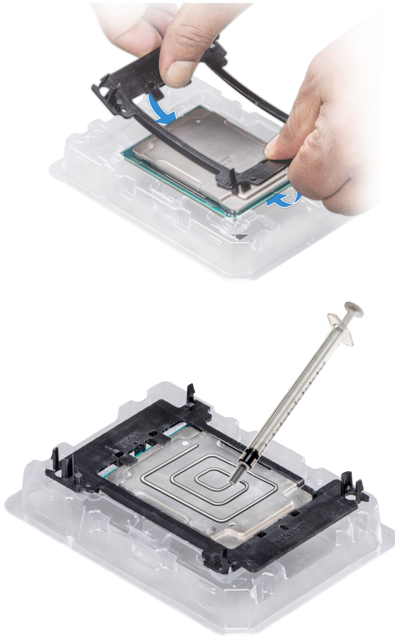
Figure 43. Applying thermal grease on top of the processor
