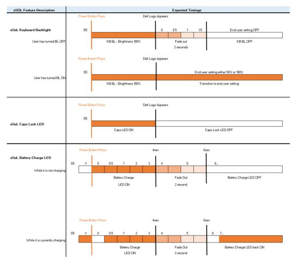
Power button with fingerprint reader will have no LED and will leverage the available LED's in the system to provide indication of the system status
